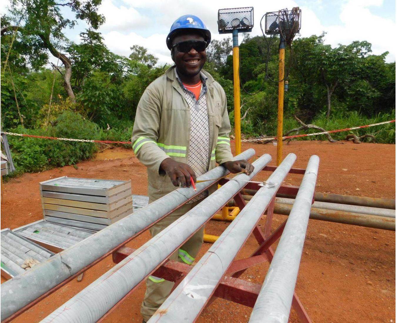
A geological technician measures the rock quality at exploration drill hole DD1319, west of the current Kakula West Discovery area.
