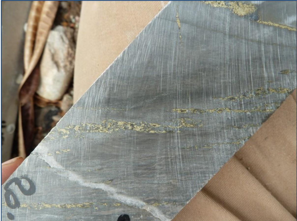
Figure 7.25 Blebbly and Disseminated Chalcopyrite in Série Récurrente Siltstone at 148 m in Drillhole KPU074. Both Mineralisation and Bedding are Deformed by Parasitic Folds
