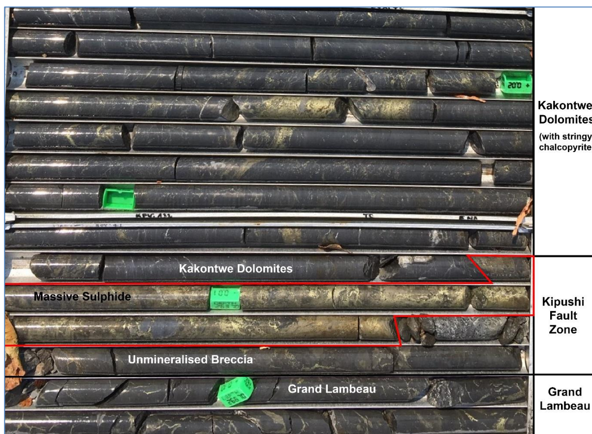
Figure 7.21 Fault Zone Copper Mineralisation Extending into the Middle Kakontwe Dolomites from Drillhole KPU132
