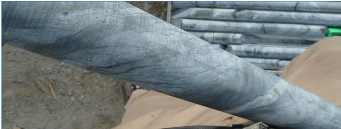
Figure 7.6 Interbedded Dolomite-shale/Siltstone Unit in the Upper Kakontwe Formation at 153 m in KPU070 (hole orientation -35 to 125). Bedding Dips Steeply to North-North-West (here in proximity to Kipushi Fault Zone) and is cut by a Steep East-West Cleavage. Core is Positioned such that the Image Represents a Plan View with North to the top
