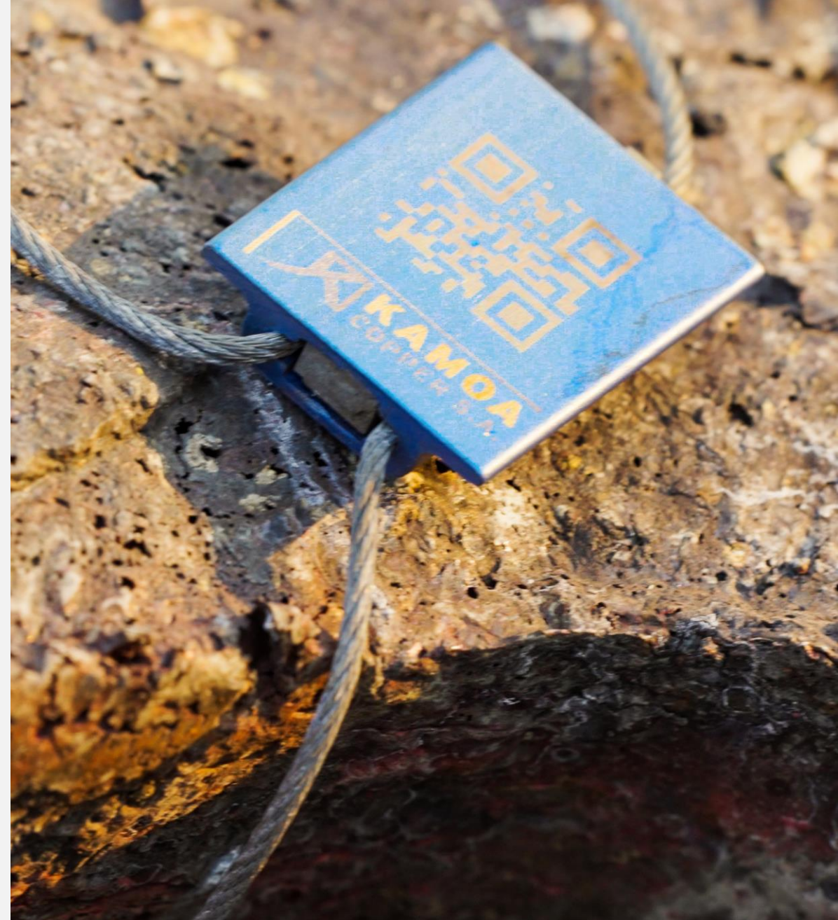
A blister copper ingot produced at the Lualaba Copper Smelter near Kolwezi, containing approximately 99% copper, ready for export to international markets.
