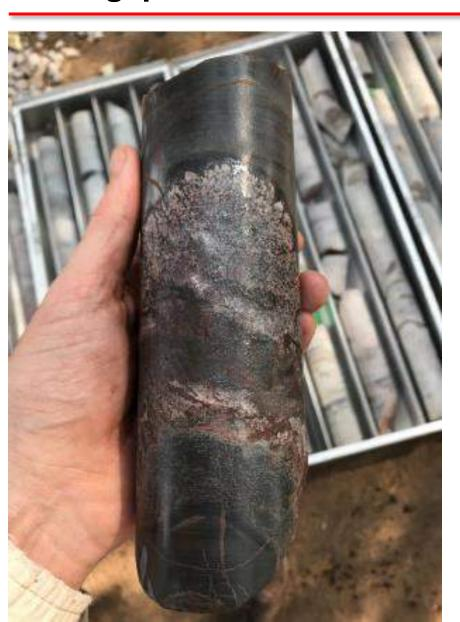
Chalcocite (copper sulfide, Cu2S) is opaque and dark-grey to black and is 80% copper by weight).
