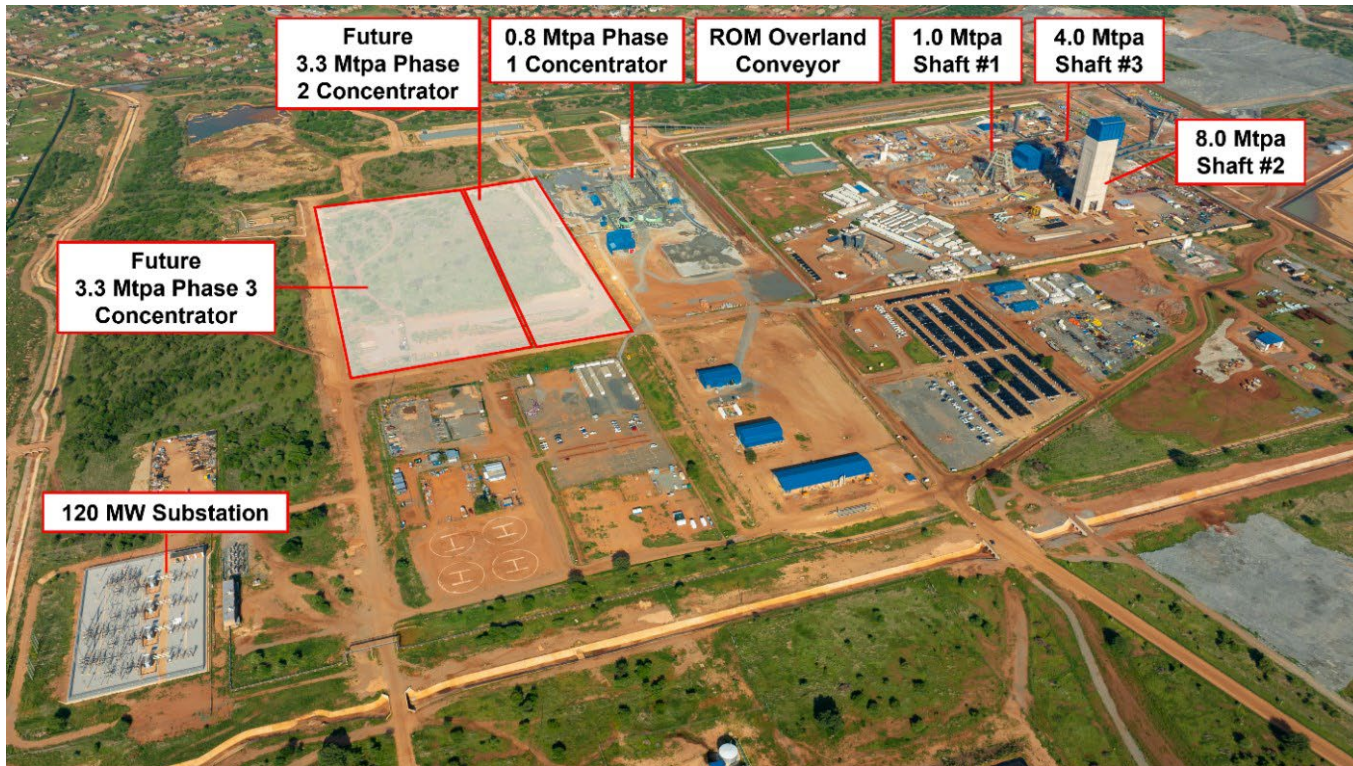
Photo: Aerial view of the Platreef Mine site, showing the existing surface infrastructure, as well as an outline of the locations for the future Phase 2 and 3 concentrators, adjacent to the current Phase 1 concentrator.
