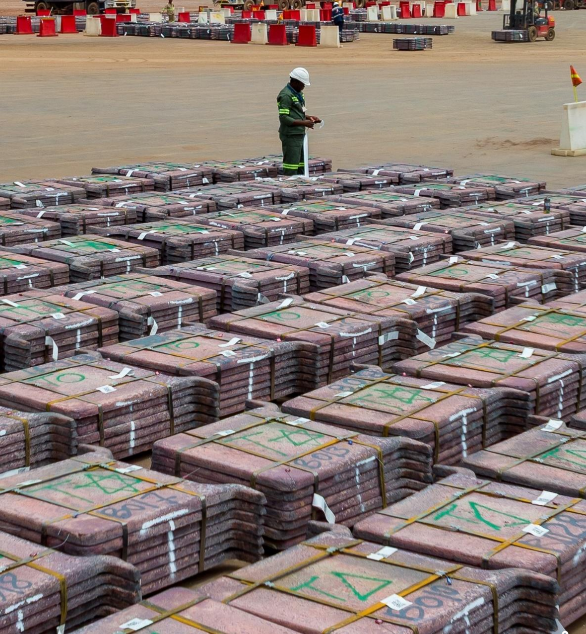
99.7%-pure copper anodes are inspected in the anode yard of the Kamoakakula smelter prior to loadout and export. The first sales of 99.7%-pure copper anodes and high-strength sulphuric acid took place in Q1 2026.
