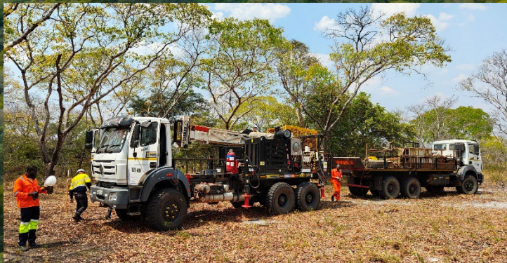
Mobilization of the diamond drill rig in April for the 12-hole stratigraphic drill program
