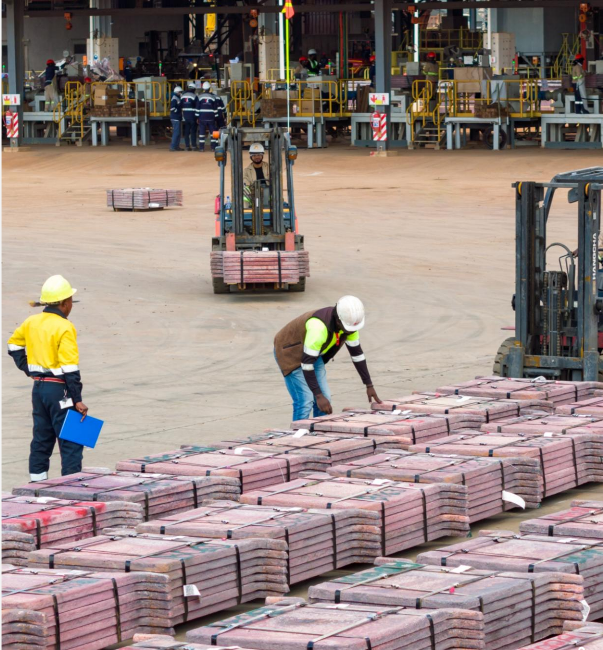
99.7%-pure copper anodes are inspected in the anode yard of the Kamoakakula smelter prior to loadout and export. First production of 99.7%-pure copper anodes commenced in late Q4 2025.
