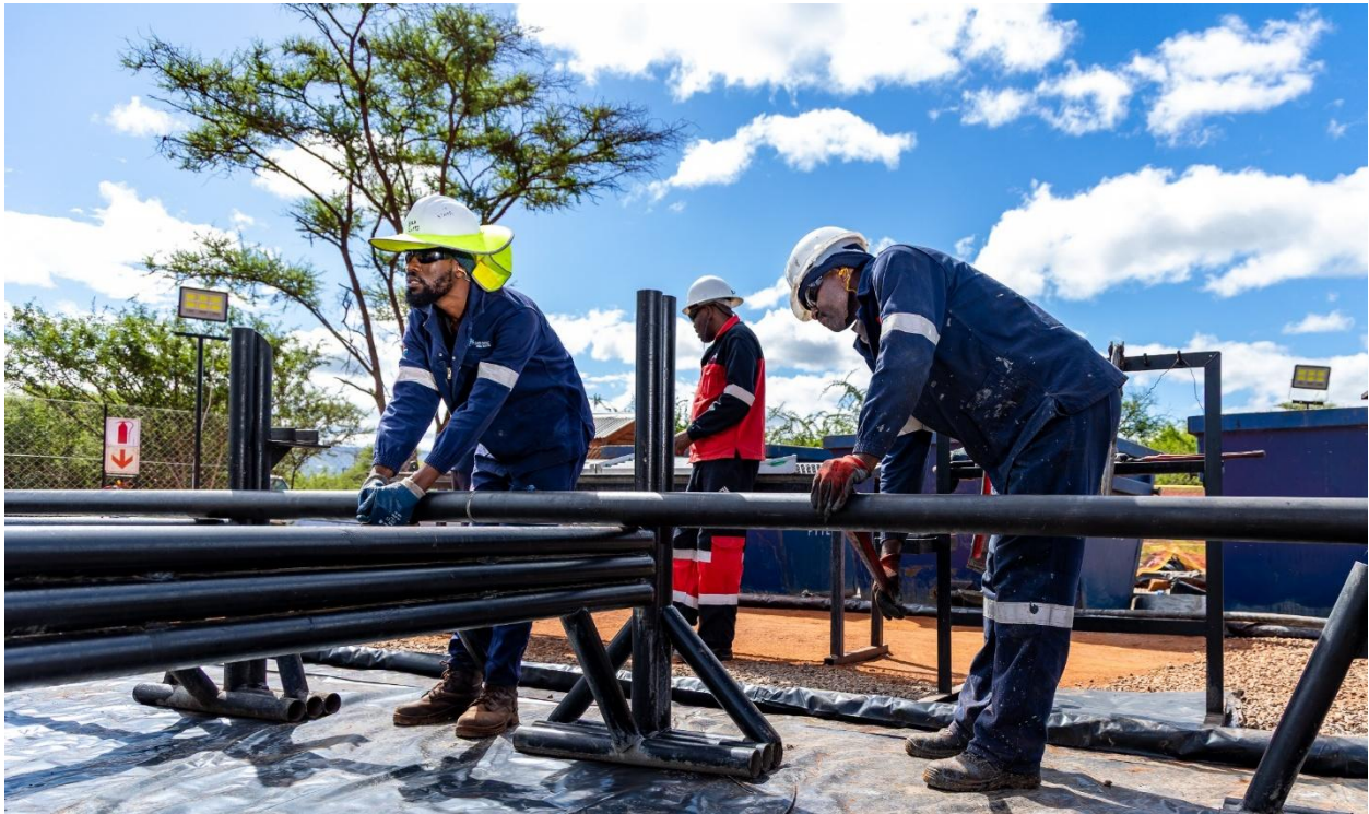
(L-R) Guvet Mashamaite, Ernest Mbedzi, and David Maluleka (back) connecting drill rods at the Mokopane Feeder drill site.
