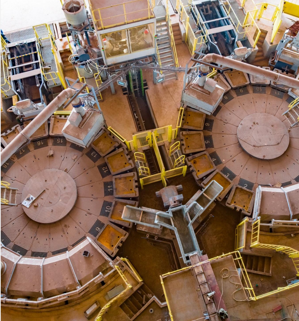
Looking down on the casting wheels inside Kamoakakula's recently completed 500,000-tonnes-per-annum copper smelter. Production of 99.7%-pure copper anodes is expected to commence in Q4 2025.
