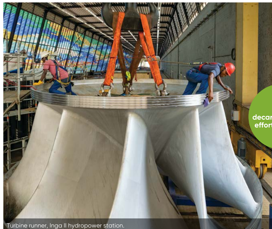
Turbine runner, Inga II hydropower station.
