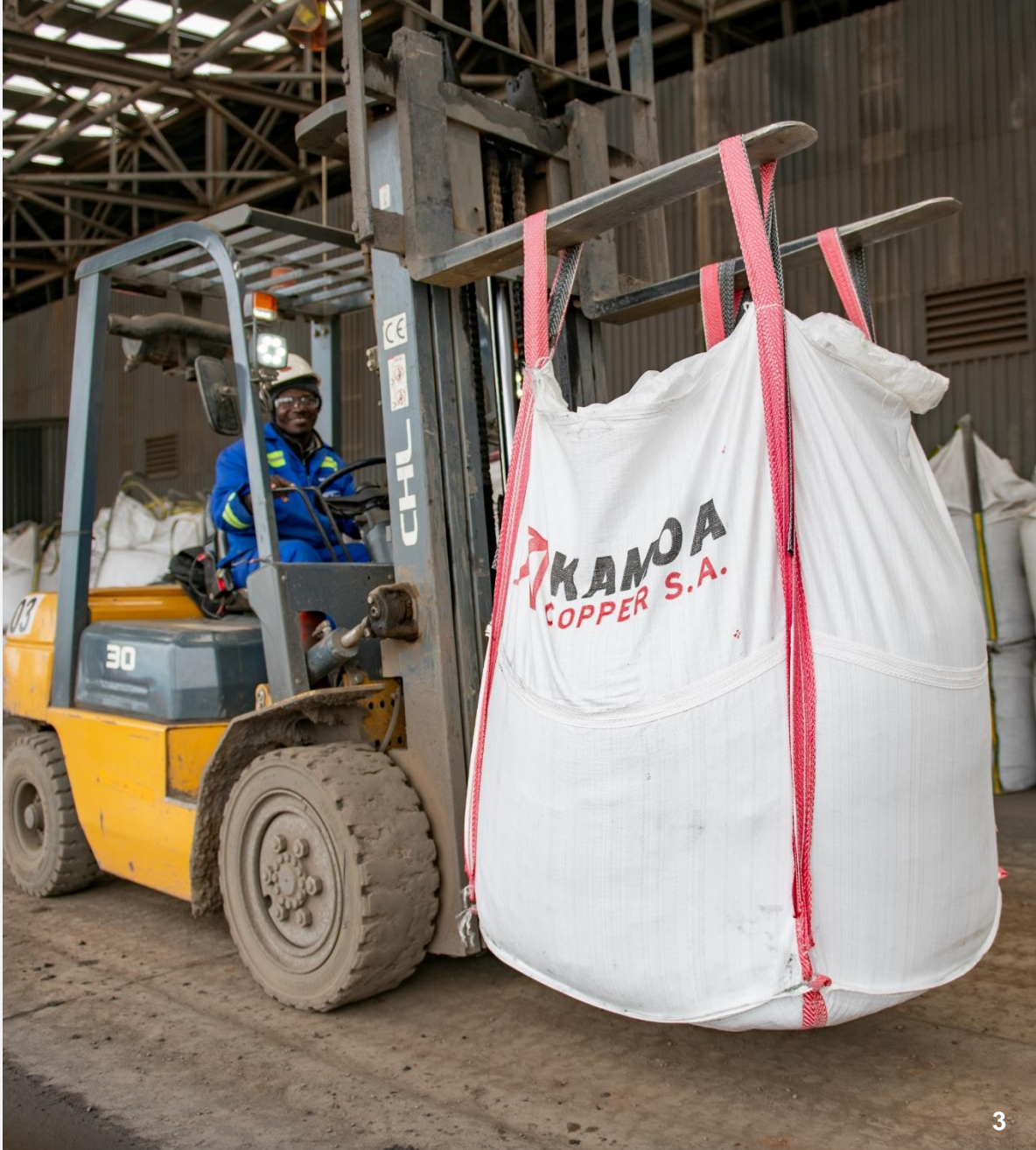
2-tonne bag of copper concentrate ready for export. Kamoa-Kakula's concentrate is one of the highest grade in the world, at approximately 50% contained copper. It is currently shipped to smelters all over the world
