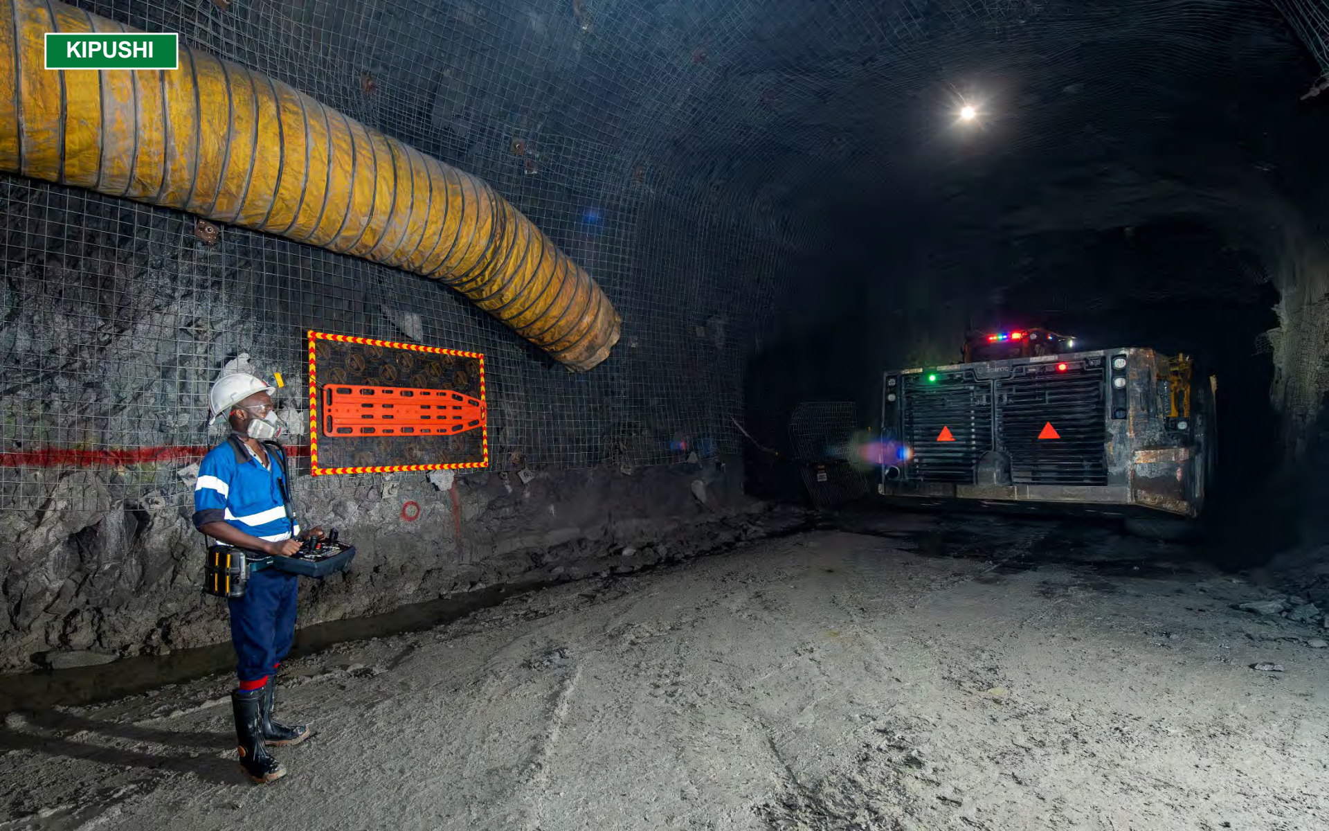
Andrew Sangra demonstrating the operation of a remote-controlled loader.
