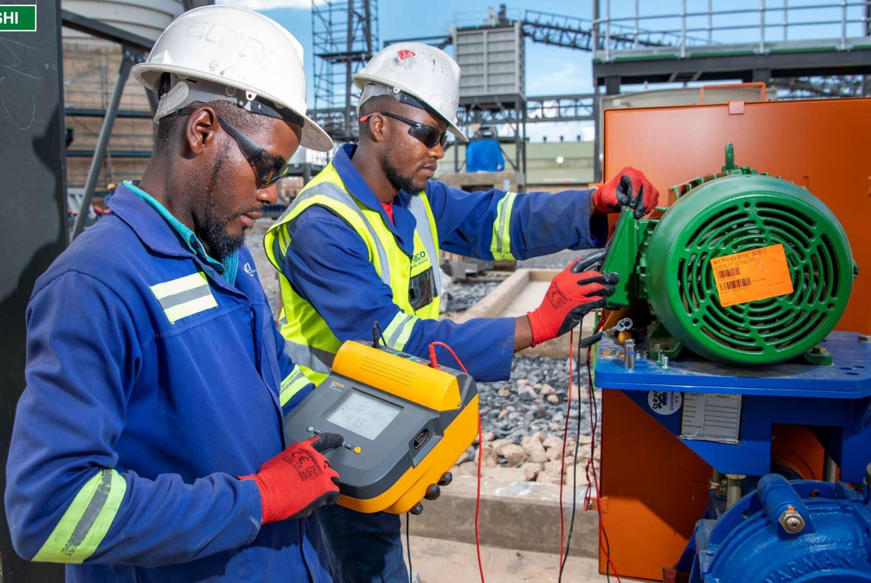
(L-R) Gloire Kumwimba and Mojej Mbuya, Electrical Quality Controllers of Panaco SARL, conducting electrical testing of a motor prior to installation.
