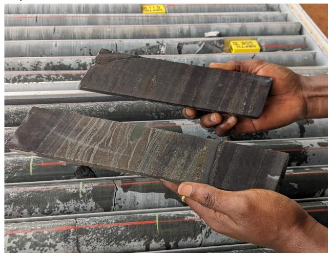
Core boxes from the diamond core drilling of the Makoko and Kiala deposit, alongside previously drilled Kakula core for comparison.
