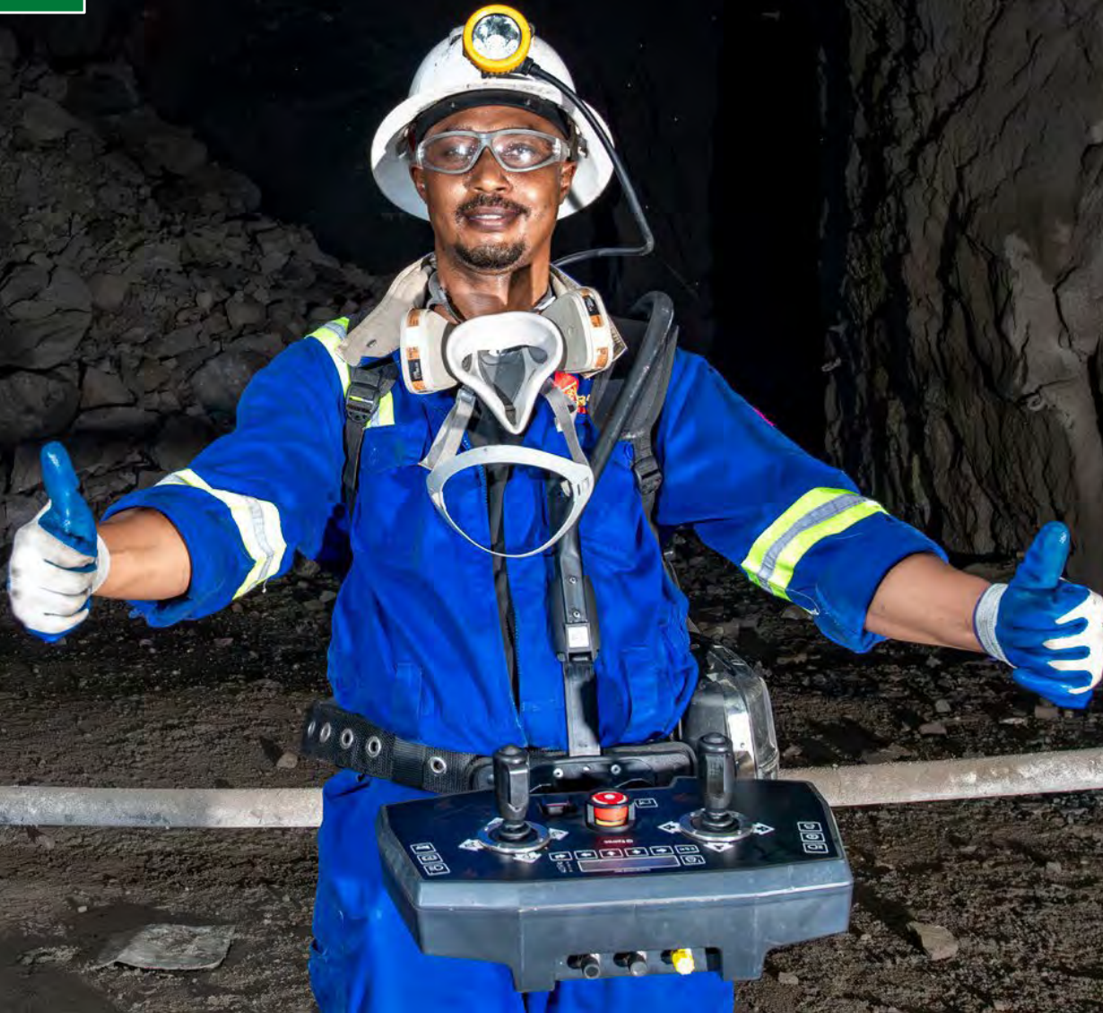
Serge Ngij Ankaz (ST14 - Operator) demonstrates how to operate the remote stope loading controls.
