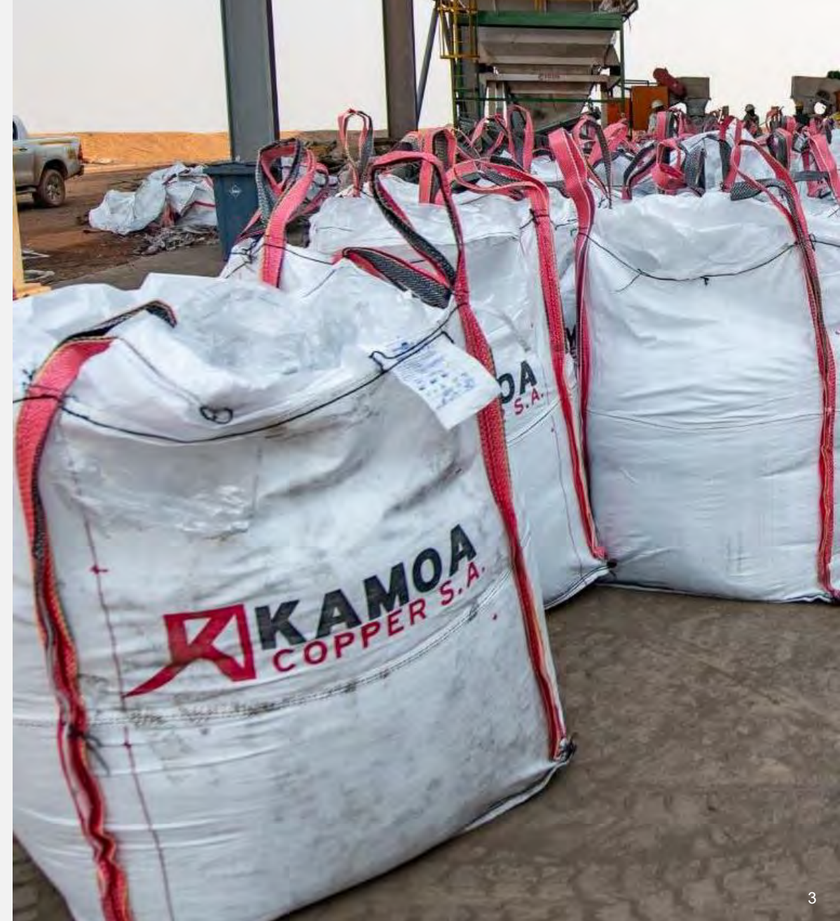
2 tonne bags of copper concentrate ready for export. Kamoakakula's concentrate is some of the highest grade in the world, at approximately 50% contained copper. It is currently shipped to smelters all over the world
