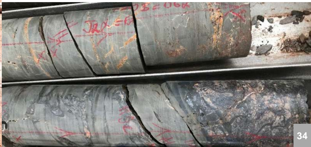
Below: Massive and bedded chalcocite within siltstone.
