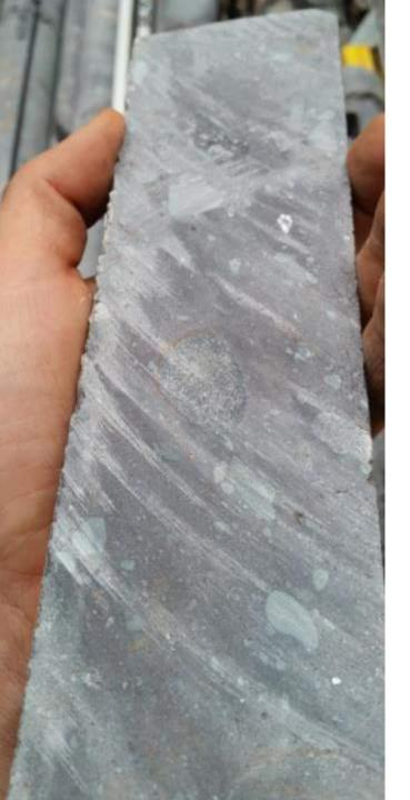
Core from Kakula drill hole DD1016, which intersected 8.75 metres (true width) of 9.84% copper at a 3.0% copper cut-off, beginning at a downhole depth of 362.0 metres.
