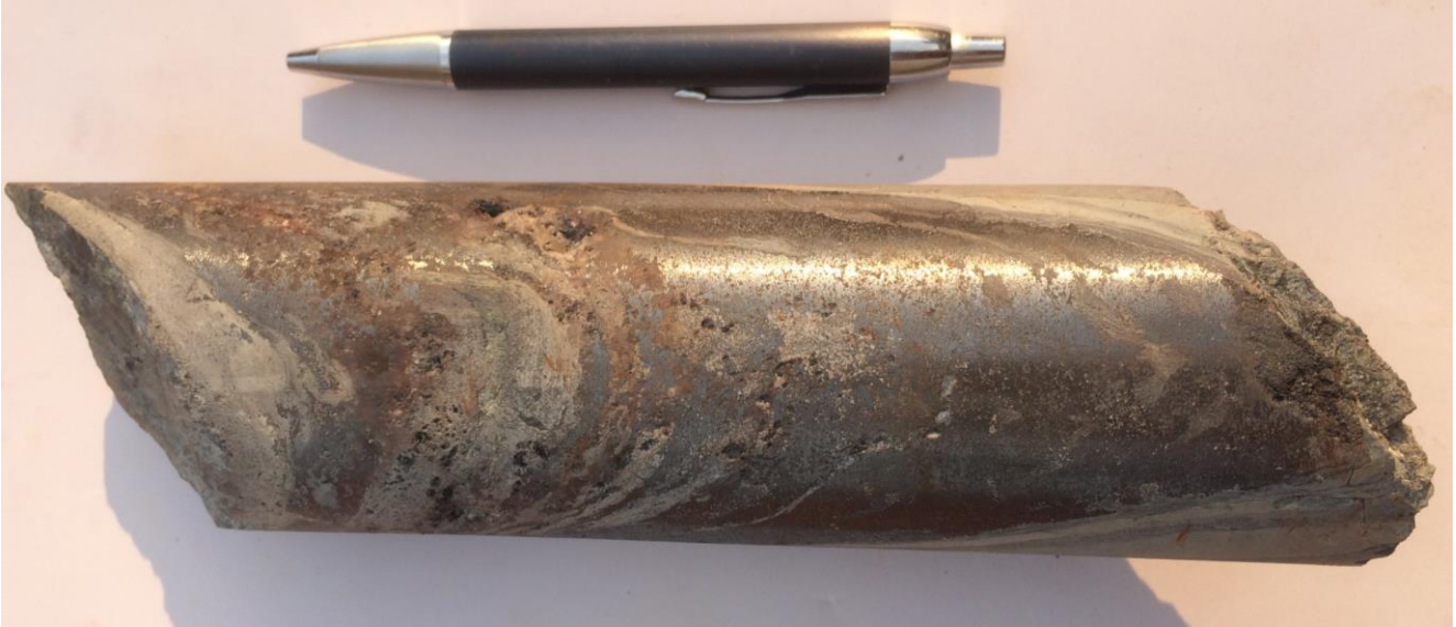
Figure 3. Intercept from DD1055, an in-fill hole in the north-west of the Kakula Discovery, with massive chalcocite at a depth of 347 metres (chalcocite is approximately 80% copper by weight).
