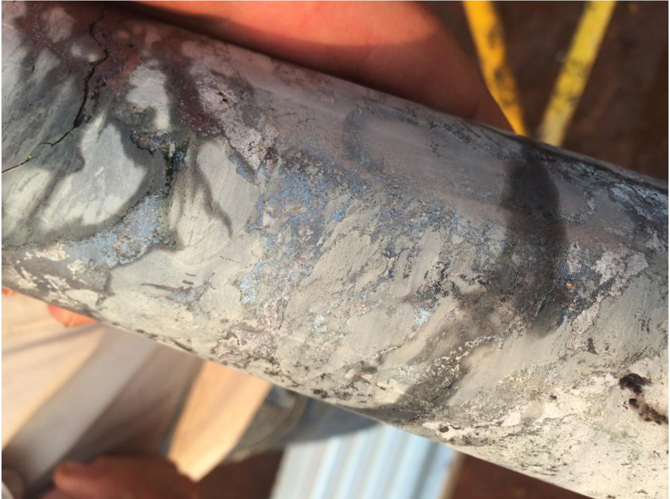
Figure 1. Drill core from DD1041 with disseminated chalcocite in diamictite at a depth of 619 metres (chalcocite is approximately 80% copper by weight).
