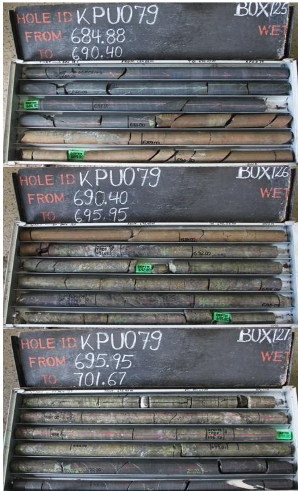
Figure 7: KPU079 showing the deepest recorded intersection of mineralization at Kipushi. Massive sphalerite from 688.1 to 691.53 metres and massive chalcopyrite with pyrite and calcite veining from 691.53 to 699.94 metres – a vertical depth of 1,825 metres.
