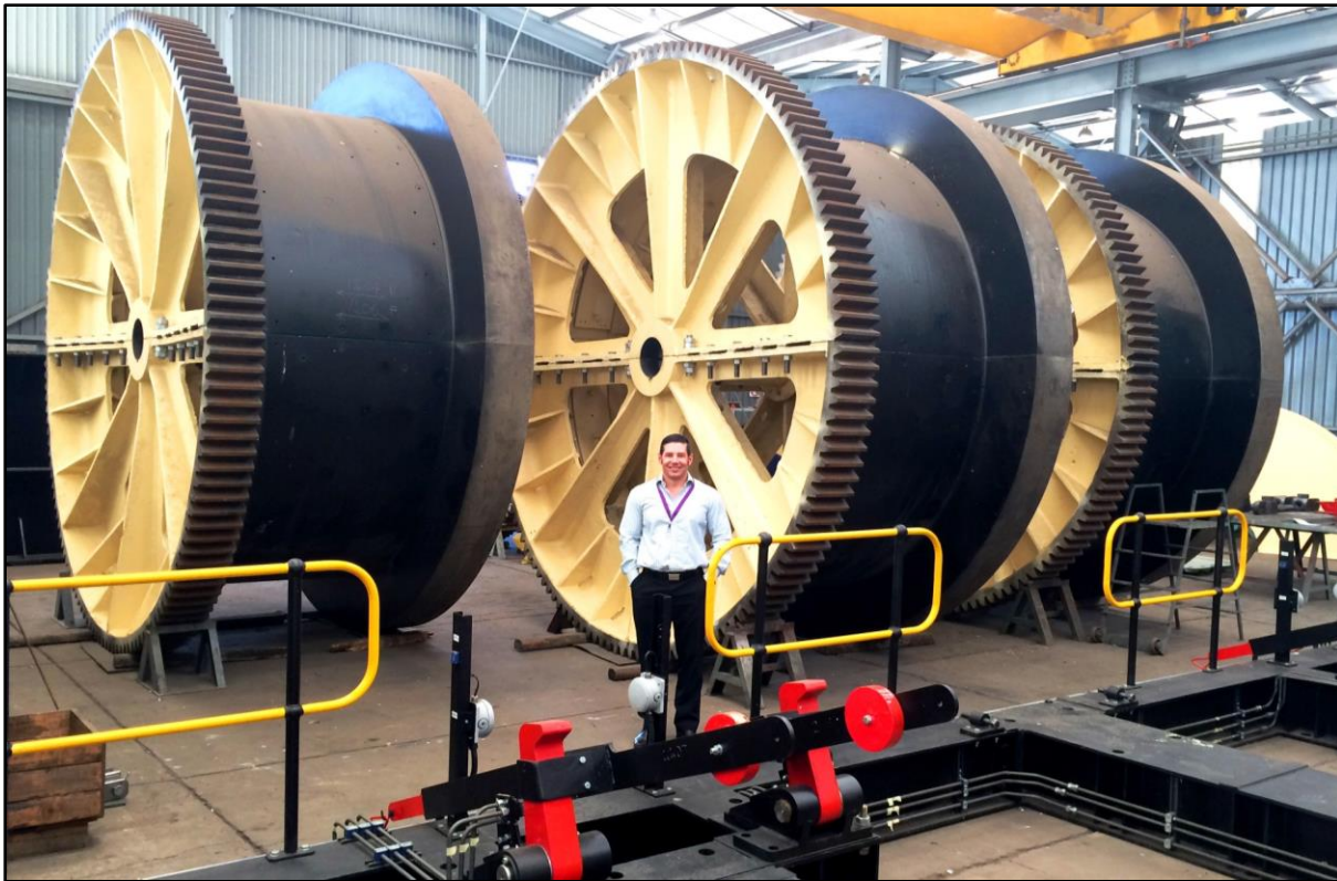
Figure 6: Refurbished winding equipment for Shaft 1.
