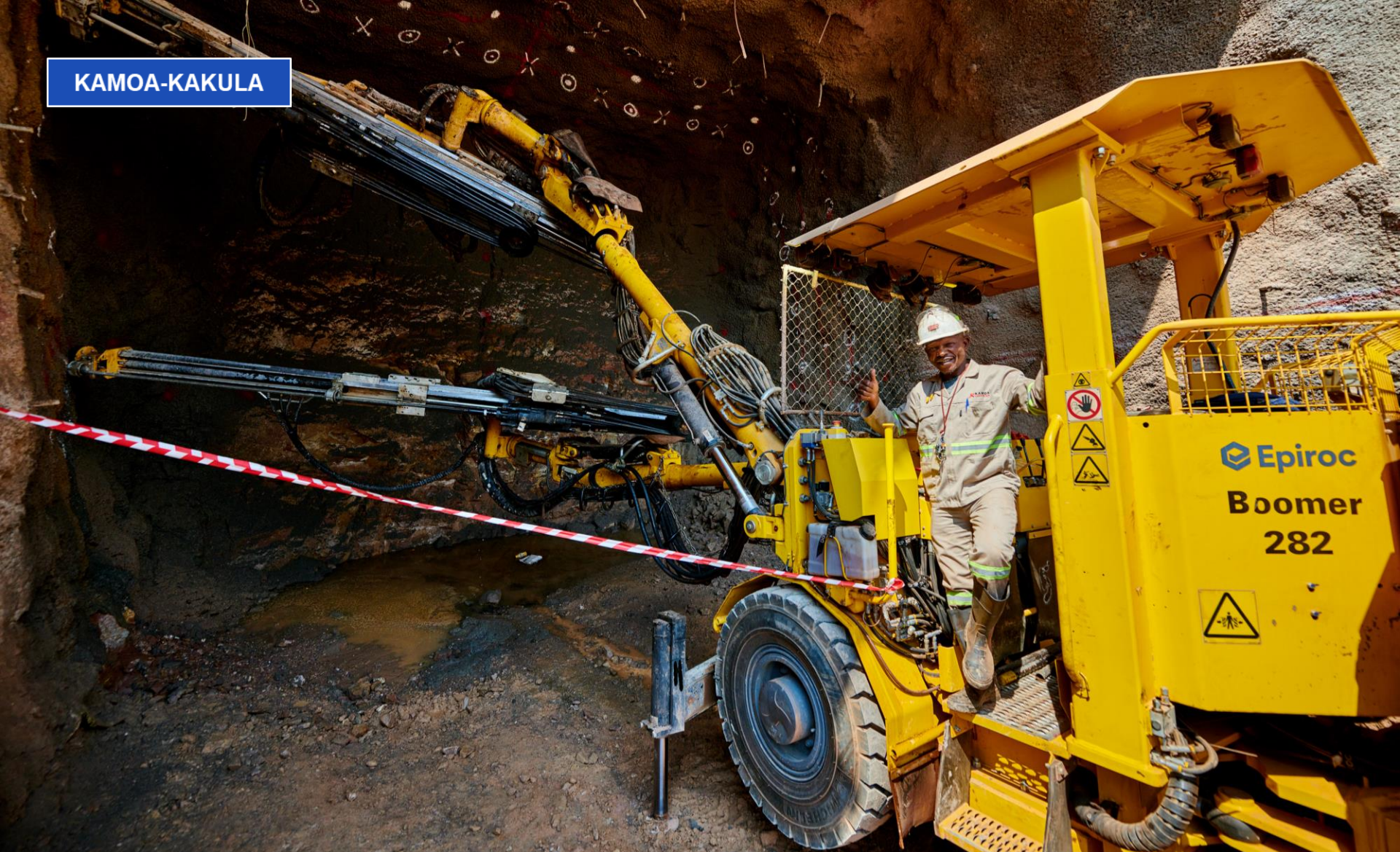
Joseph Kalenga Kabulu, Kamoa drill rig operator, drilling support holes at the Phase 3 Kamoa 1 and Kamoa 2 box cut.
