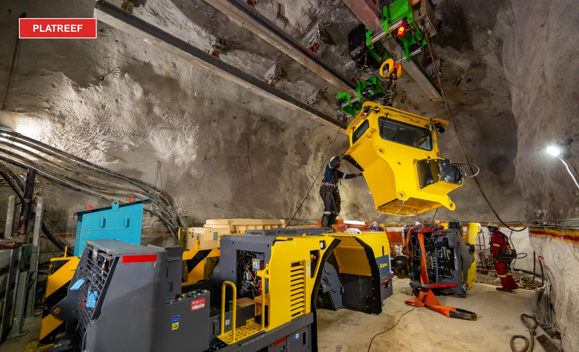
Crews assembling Ivanplats' first battery-electric underground mining vehicle, an Epiroc ST14 battery Scooptram.
