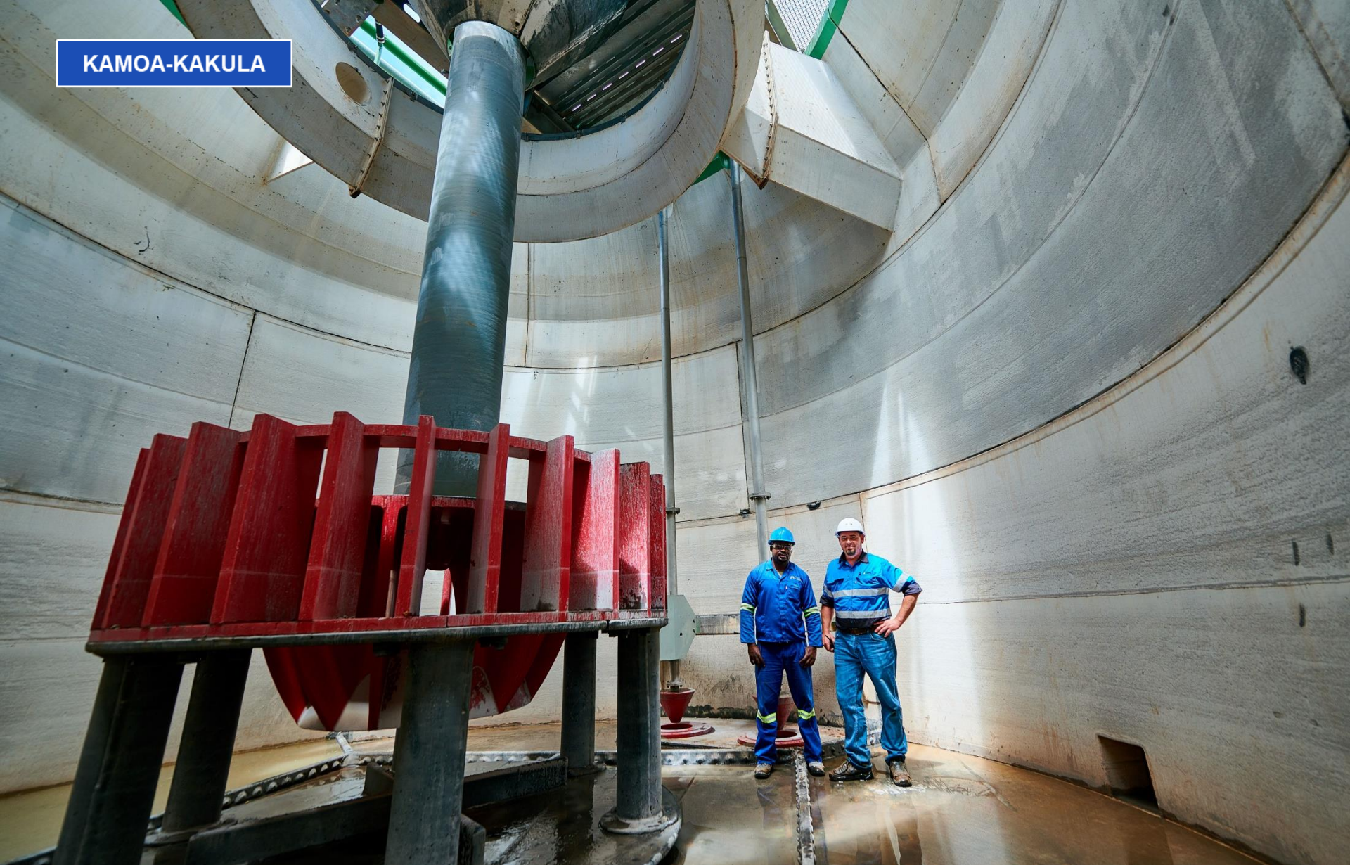
Rick Ndumba (left) and George Nel inspecting the inside of one of the Phase 2 flotation cells before commissioning begins.
