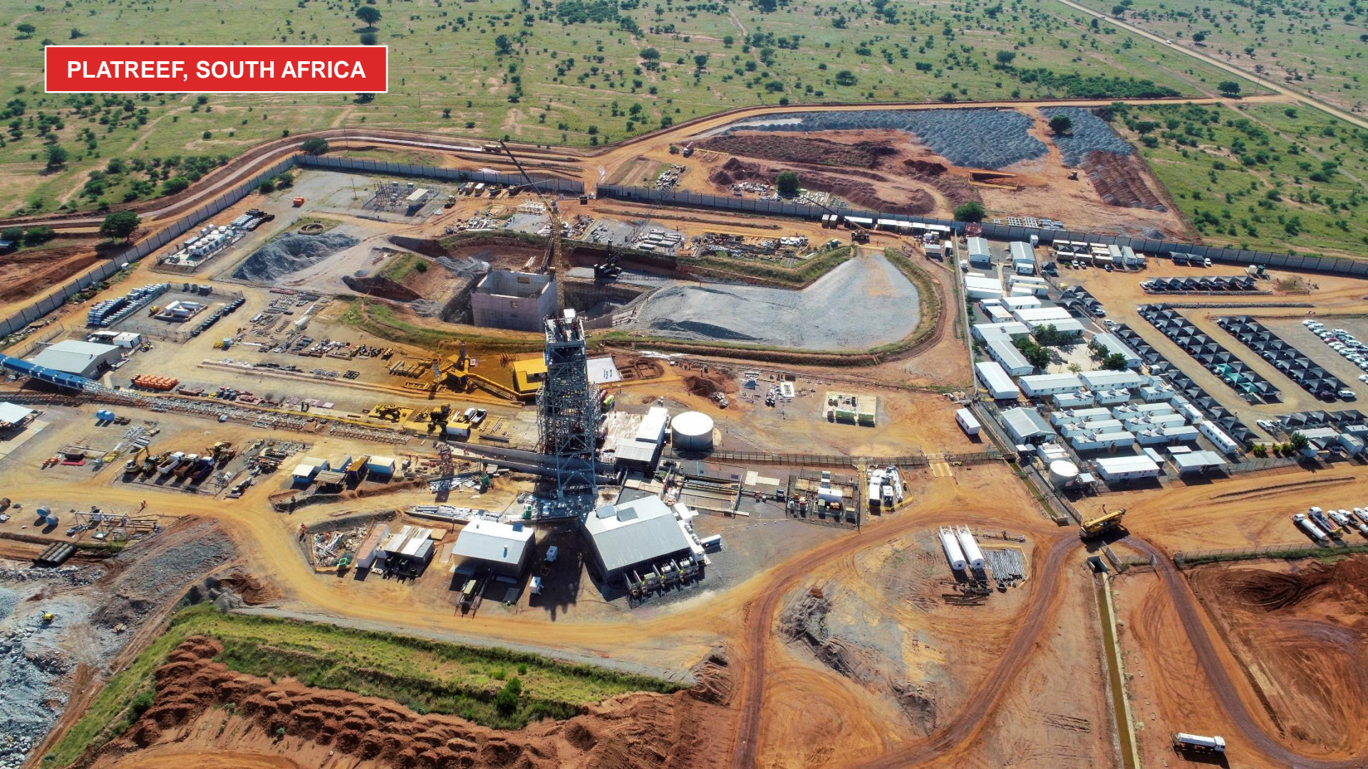
Aerial view of the Platreef Mine, with the Shaft 1 headframe in the foreground and ongoing construction of the Shaft 2 headframe immediately behind.
