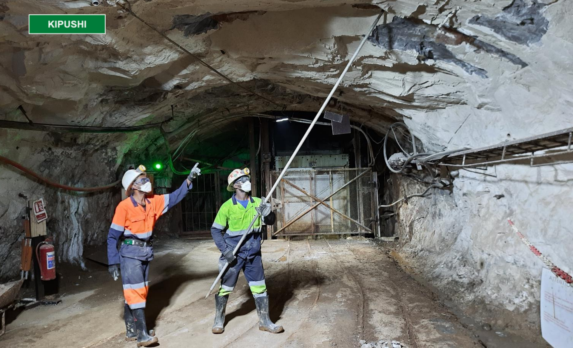
Kyunga Leya (left) and Kalenga inspecting and scaling potential loose rocks as part of Kipushi's regular preventative maintenance and safety monitoring of the mine's underground workings.
