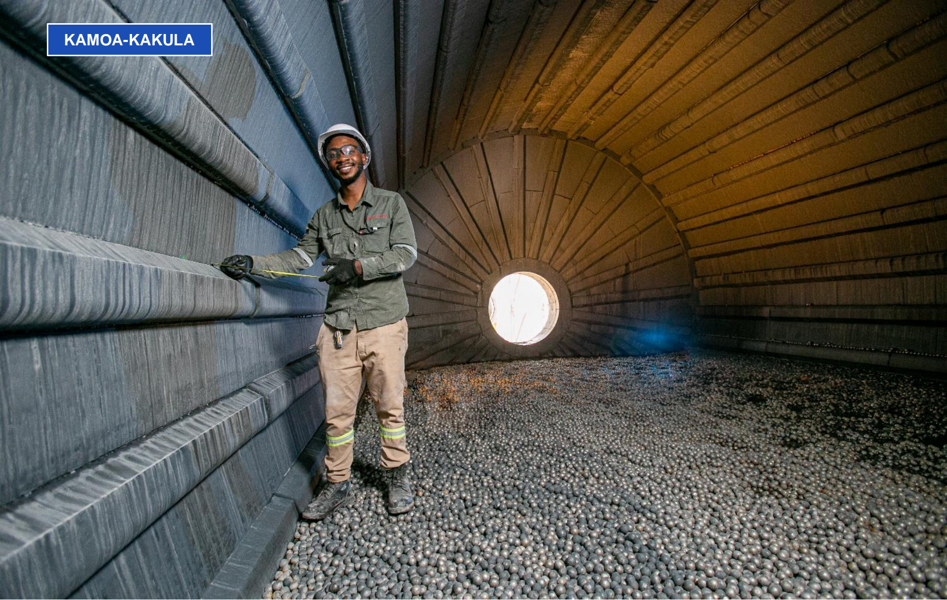
Kamoa Copper's Rodrigue Uzan measuring the wear of the rubber liners in one of two ball mills in the Phase 1 concentrator plant.
