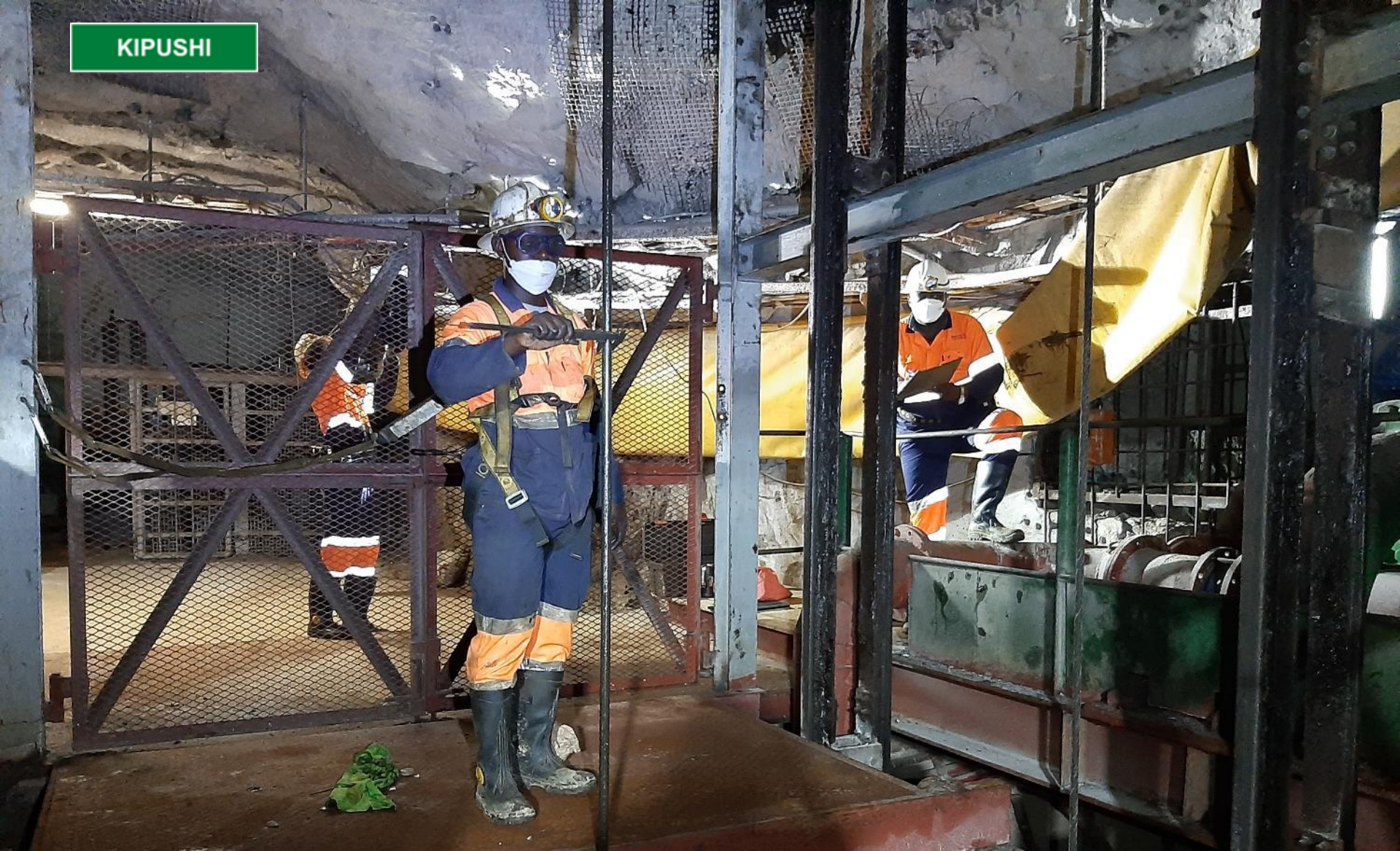
Mechanical maintenance manager Kasangula conducting monthly testing of Kipushi's Shaft 5 winder cable.
