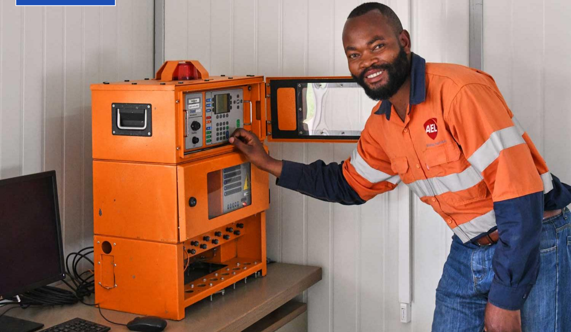
Jacques Muyumba, AEL Mining Services Engineer, programming Kakula's central blasting unit.
