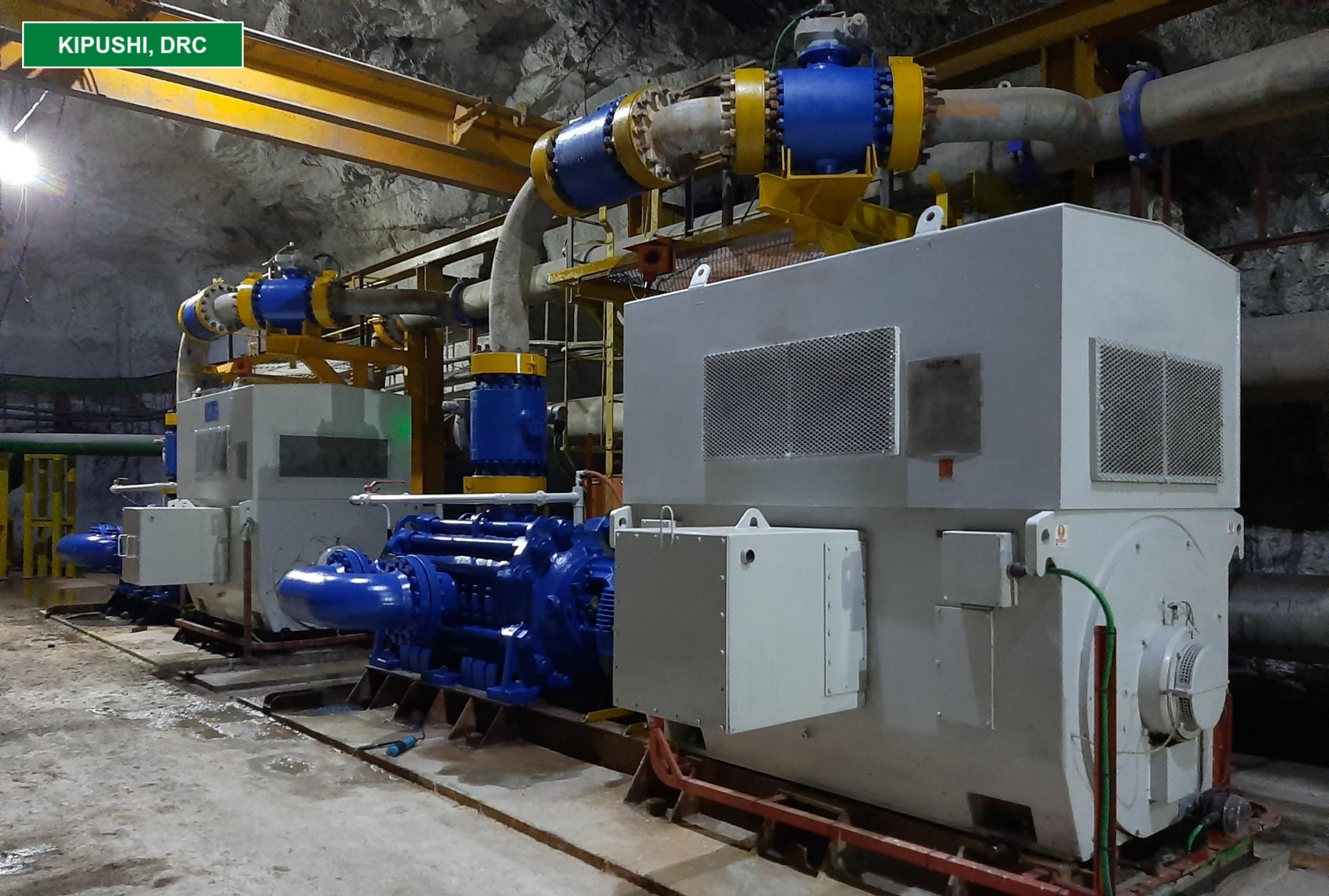
The new Grifo water pumps at Kipushi's 850-metre-level pumping station. 23
