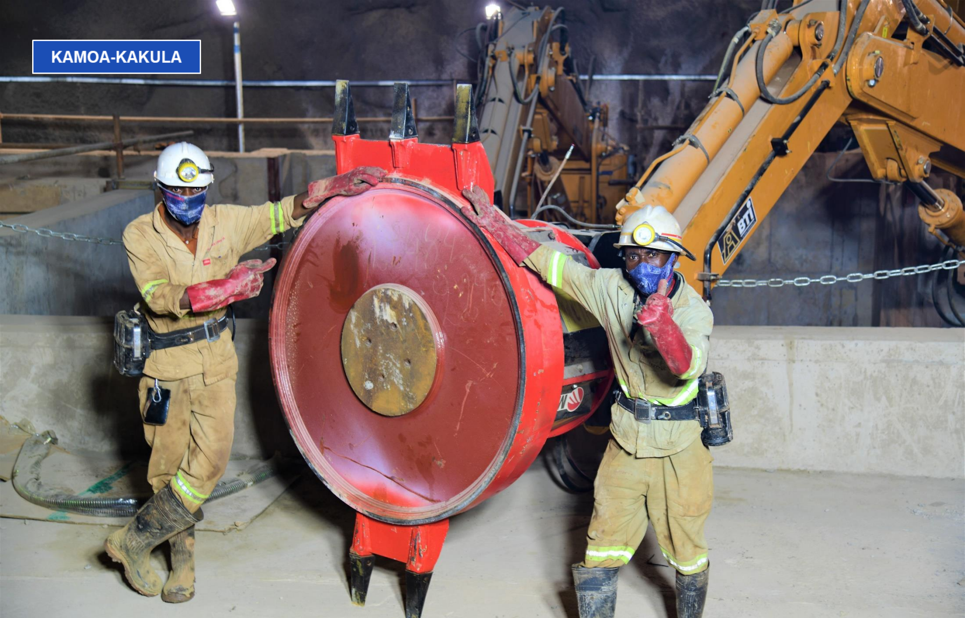
Mioi Kabinda (left) and Kifumbe Bijimba (right) with the newly-installed magnet and rock breaker at the east ore tip bin, part of the underground ore handling system at the Kakula Mine.
