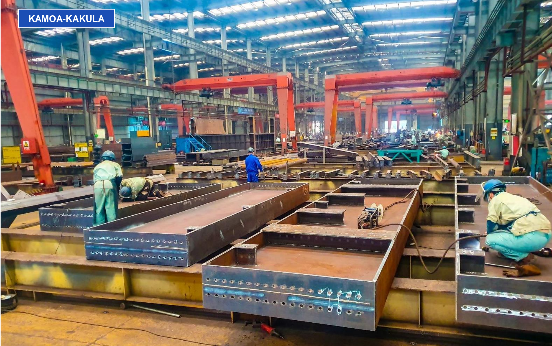
Steel support beams for Kakula's processing plant's concentrate filter being fabricated at Shanghai Modern Heavy Industries' plant in China.
