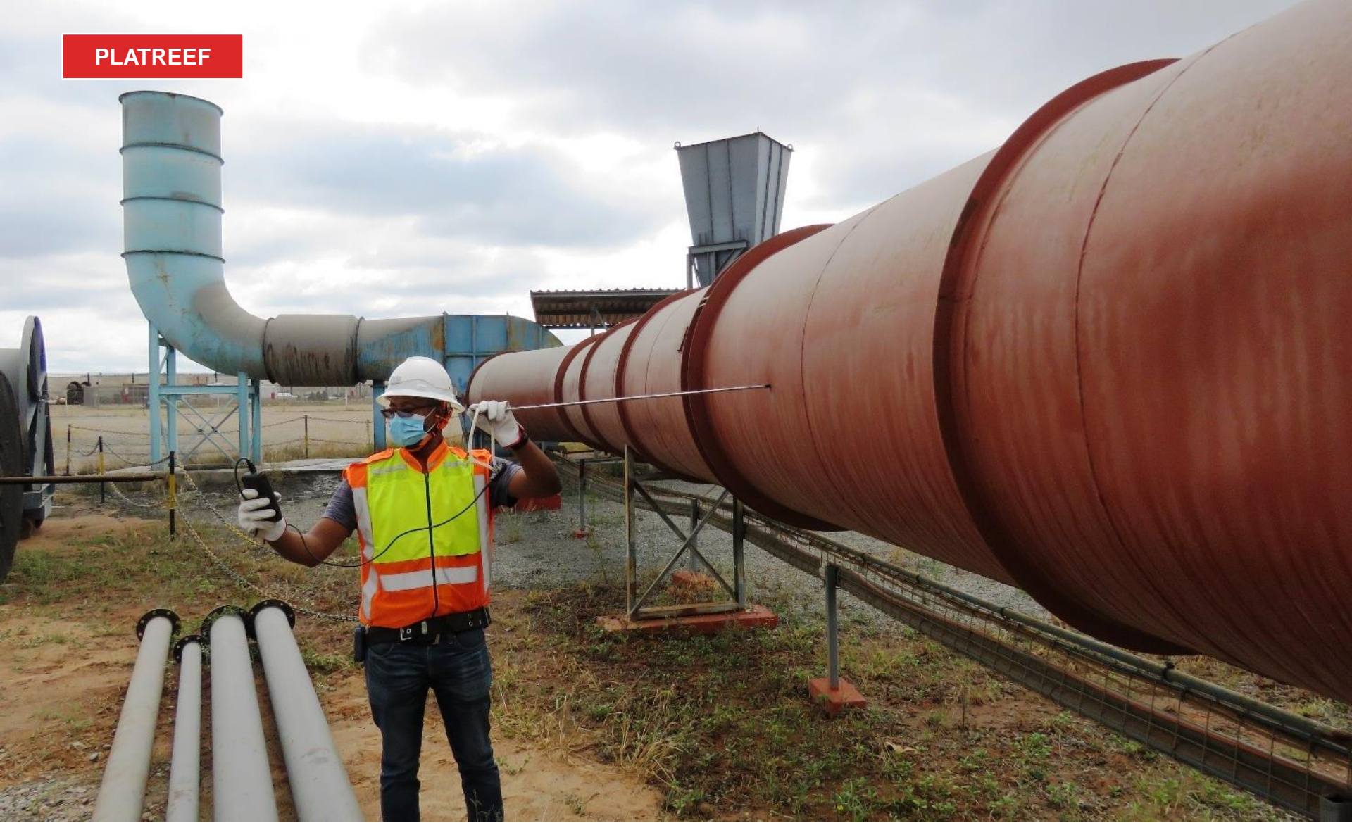
Jan Mojapelo, Ventilation Officer, measuring air flow volume from Platreef's Shaft 1 surface exhaust fan with a Pitot tube.
