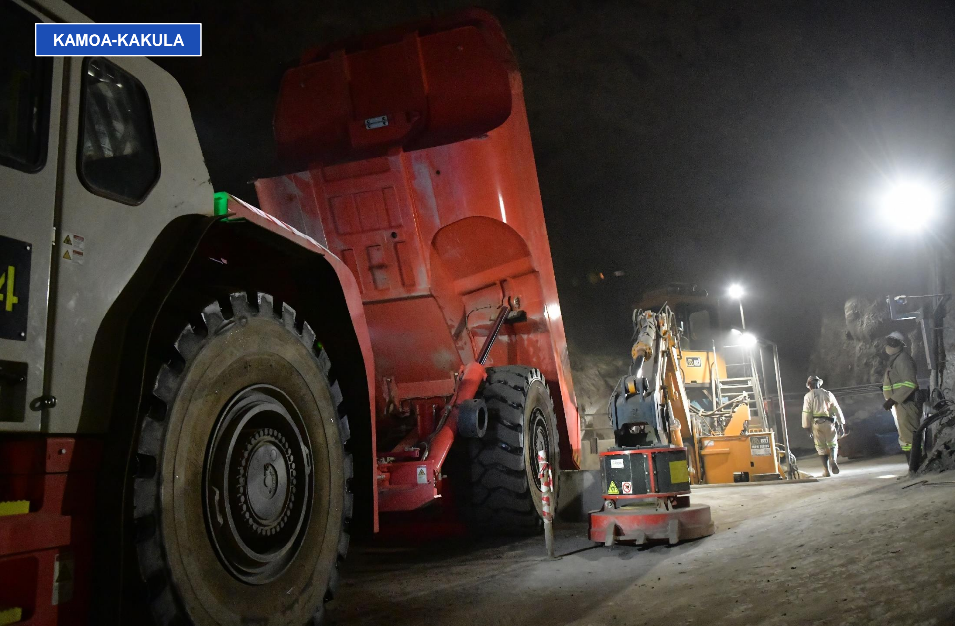
A Sandvik 63-tonne haul truck dumps its load of ore into the east tipping bin that feeds the Kakula North decline conveyor belt.
