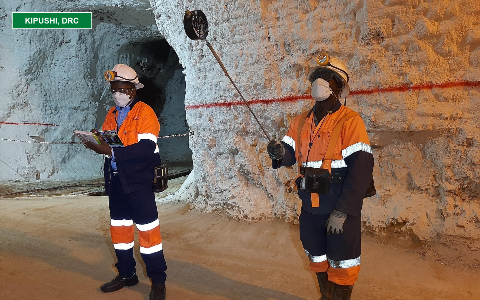
Paul Ilunga Dikwenda, Underground Manager (left), and Mbiya Kabongo, Ventilation Officer (right), conducting the monthly ventilation audit on Kipushi's 1,132-metre level.
