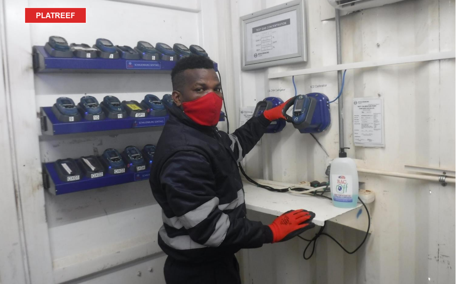
Solly Marakalala, Lampsman, calibrating the gas-detection safety instruments before the next shift commences at the Platreef Project.
