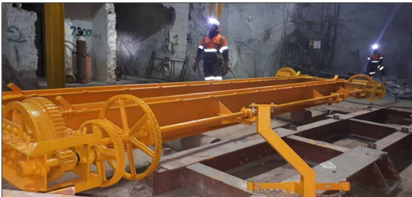
Photo: Refurbished overhead crane at Kipushi's 850-metre-level pump chamber.
