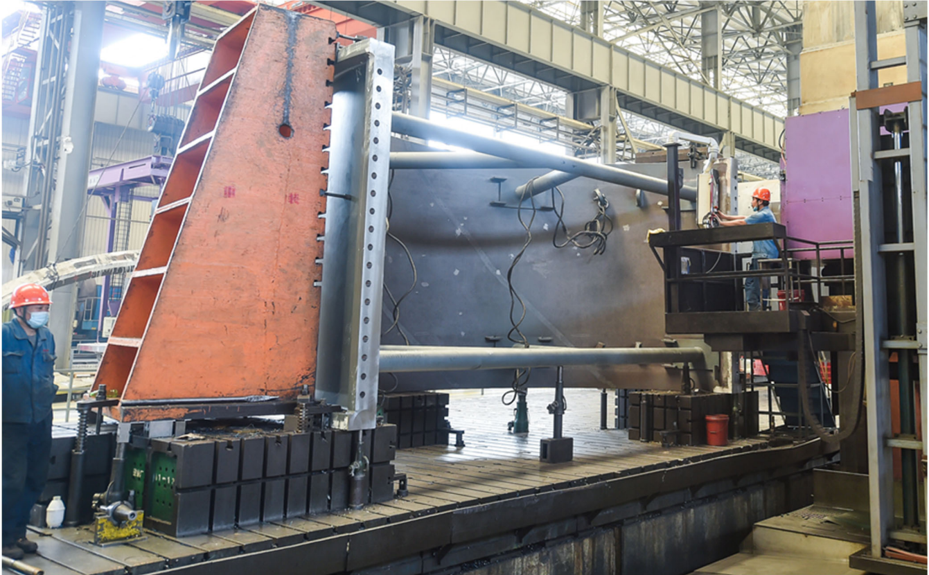
Photo: Machining of the ball mill shell at CITIC Heavy Industries' factory.
