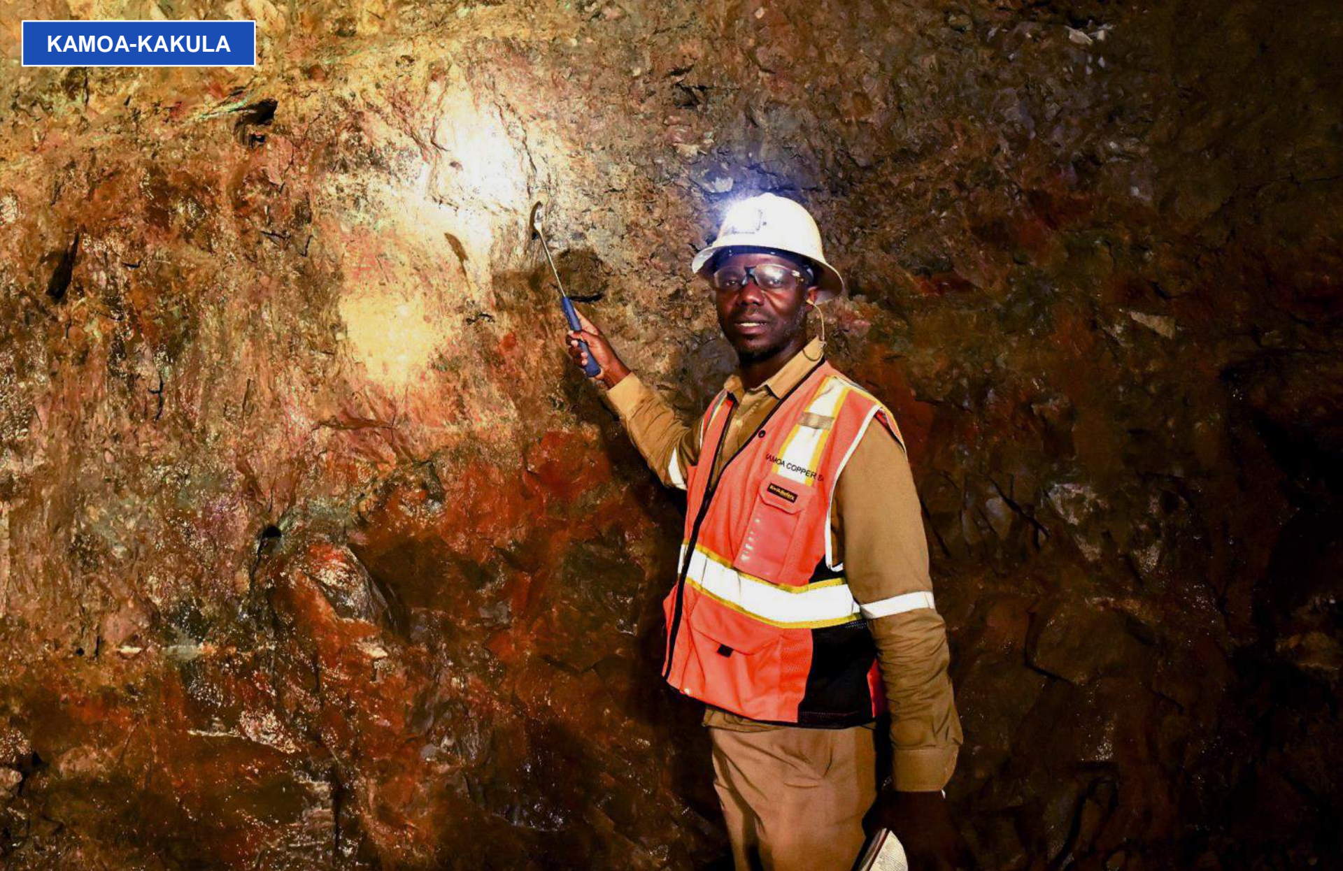
Kally Mbumba, Mine Geologist, sampling a high-grade working face in the room & pillar portion of the Kakula Mine.
