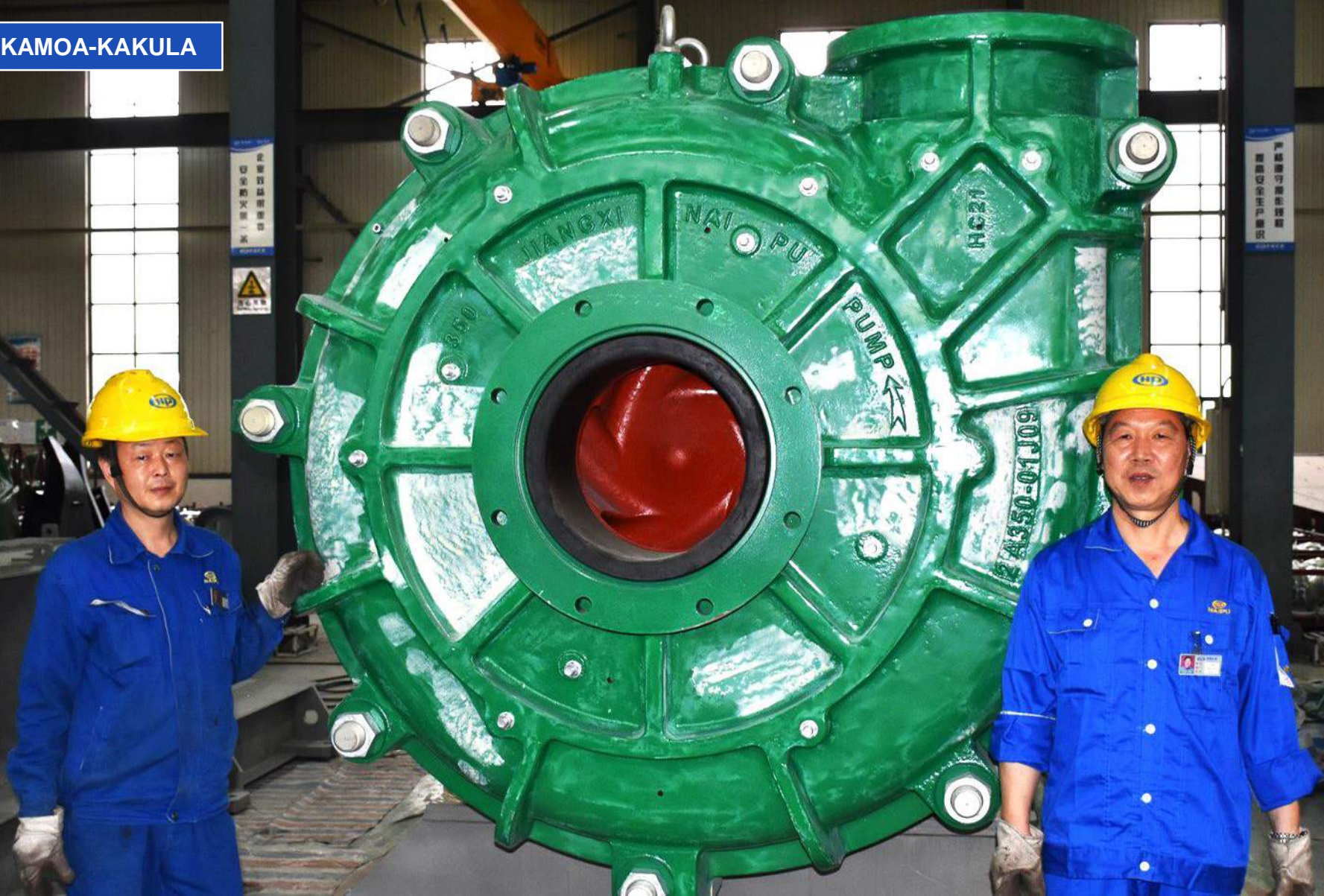
Workers at Shijiazhuang Naipu Pump Company's factory in Hebei, China, showcase a new slurry pump that will be used in Kakula's 3.8 Mtpa processing plant.
