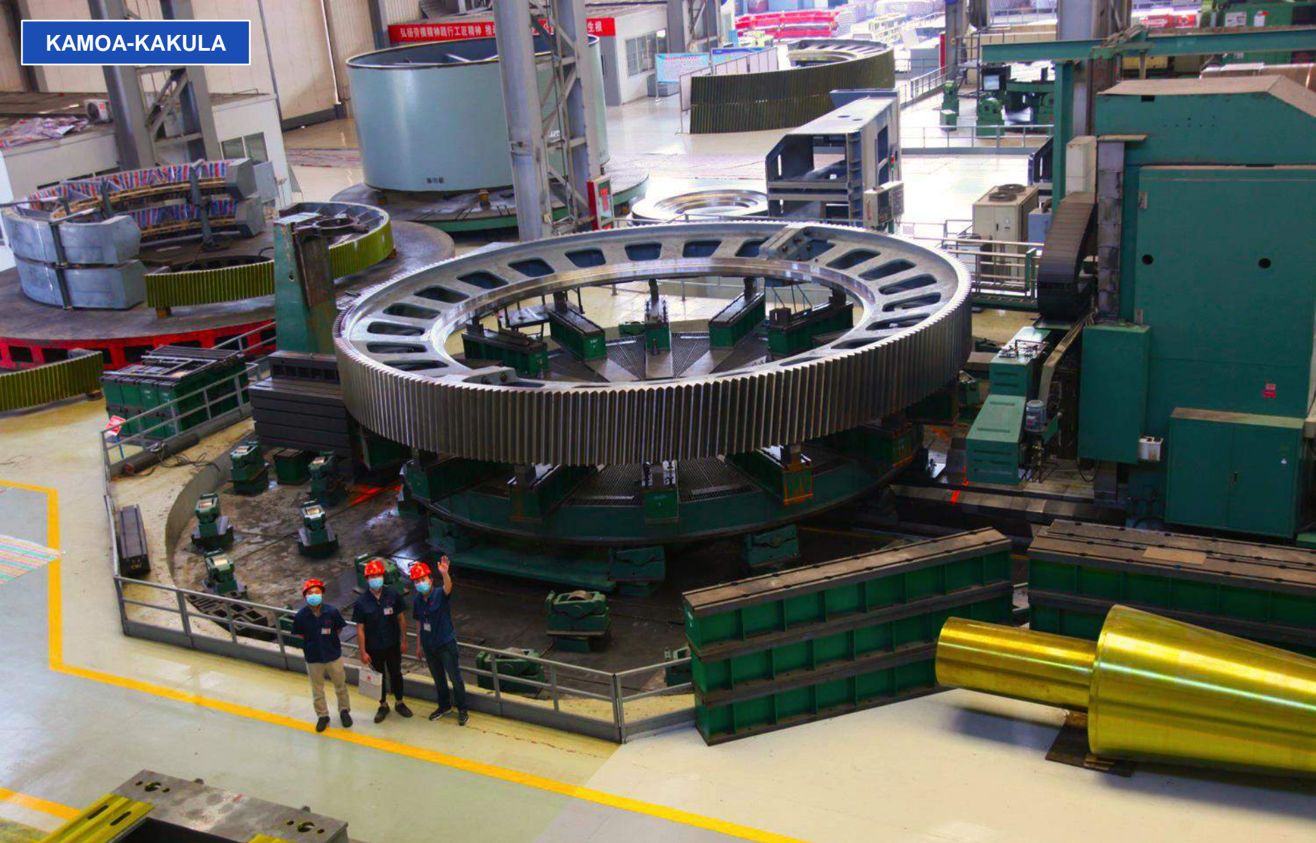
New girth gear for the Kakula processing plant's secondary ball mill recently completed at CITIC Heavy Industries' factory in Luoyang, China.
