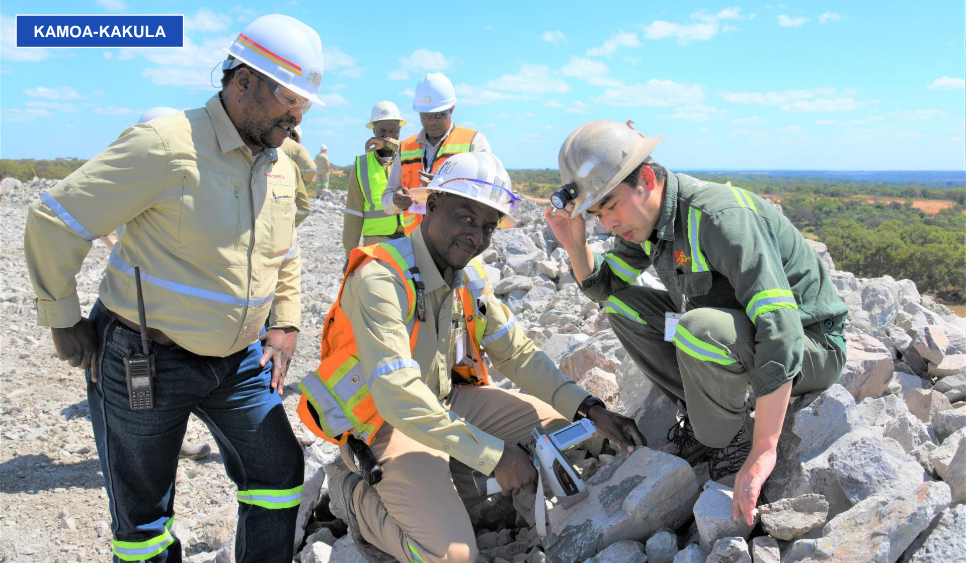
(L-R) Magloire Kashiba (Production Manager), Didier Masengo (Senior Mine Geologist) and Qiao Wei (JMMC Production Manager) examine samples of ore on the high-grade stockpile with a portable Niton analyzer (x-ray fluorescence).
