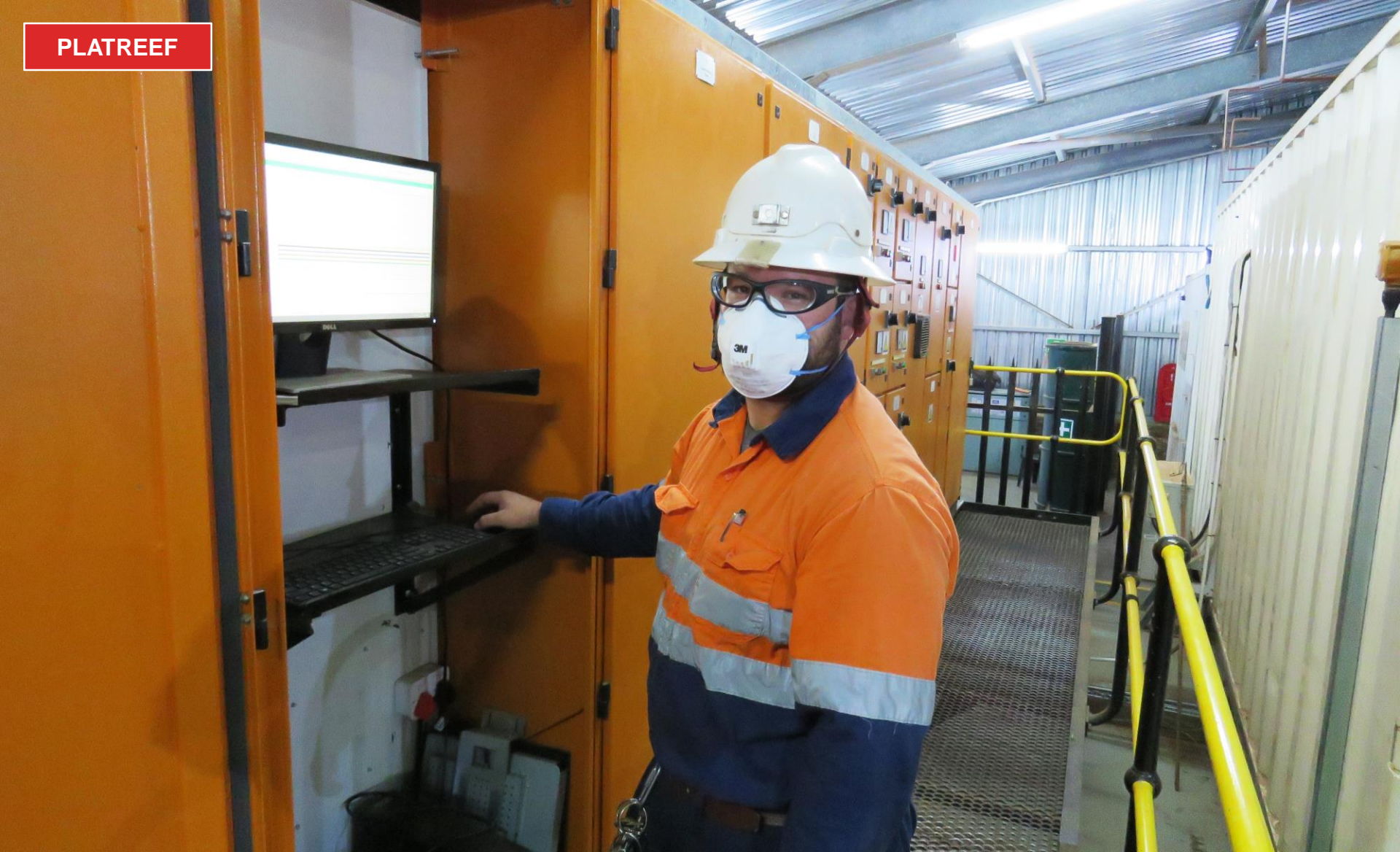
Victor Skinner (Winder Technician) analyzes the RB Recorder, which records the conveyance movements and signals within the shaft.
