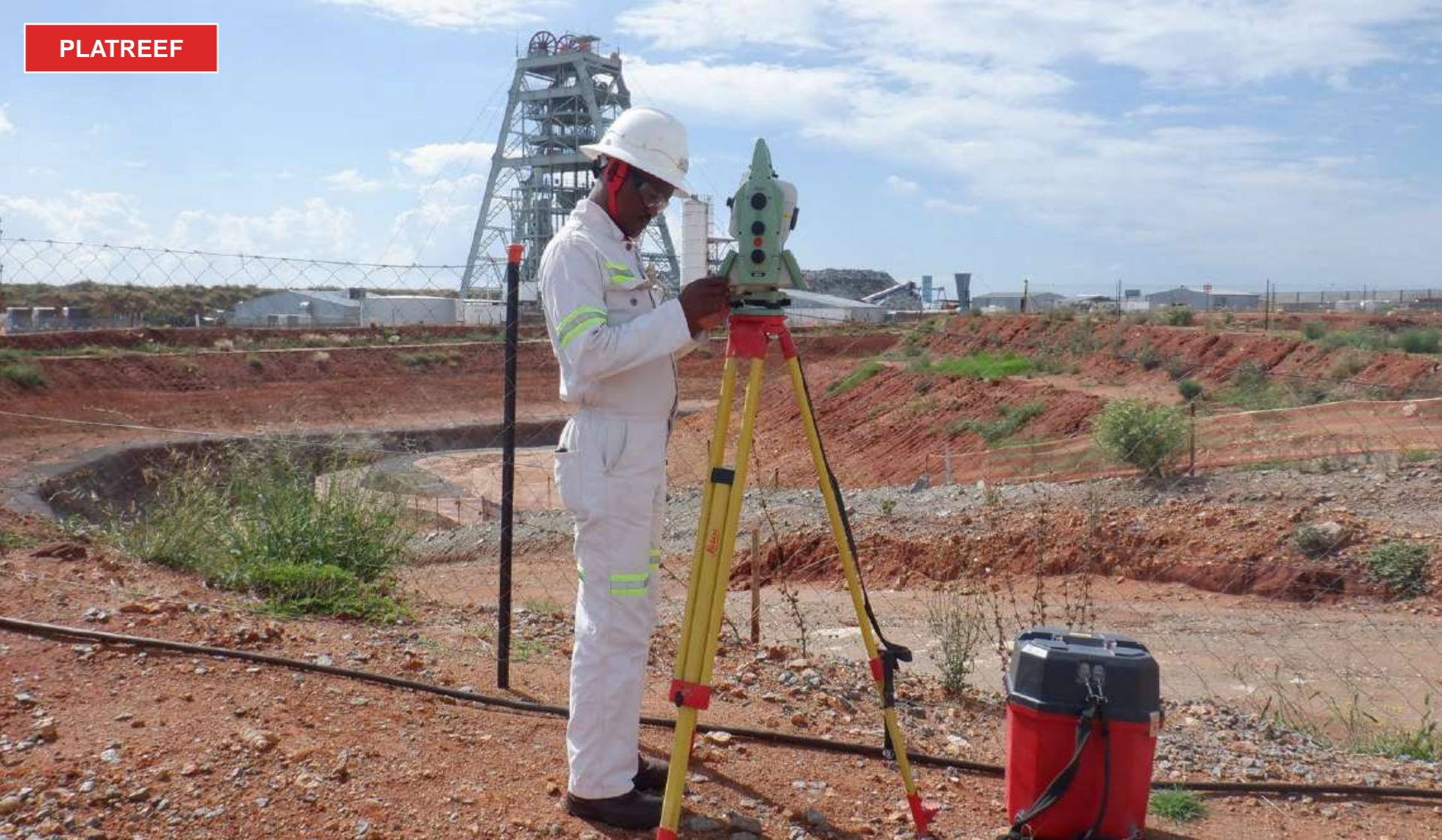
Thabiso, Surveyor, setting up his machine to conduct a scan of the Shaft 2 box cut.
