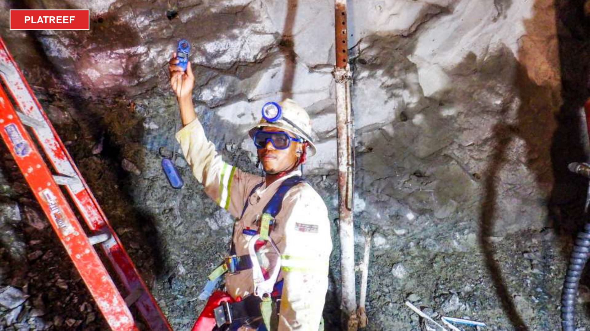
Tumelo Maselela, Miner, measuring the velocity of fresh air supplied to a development face on 950-metre-level station.
