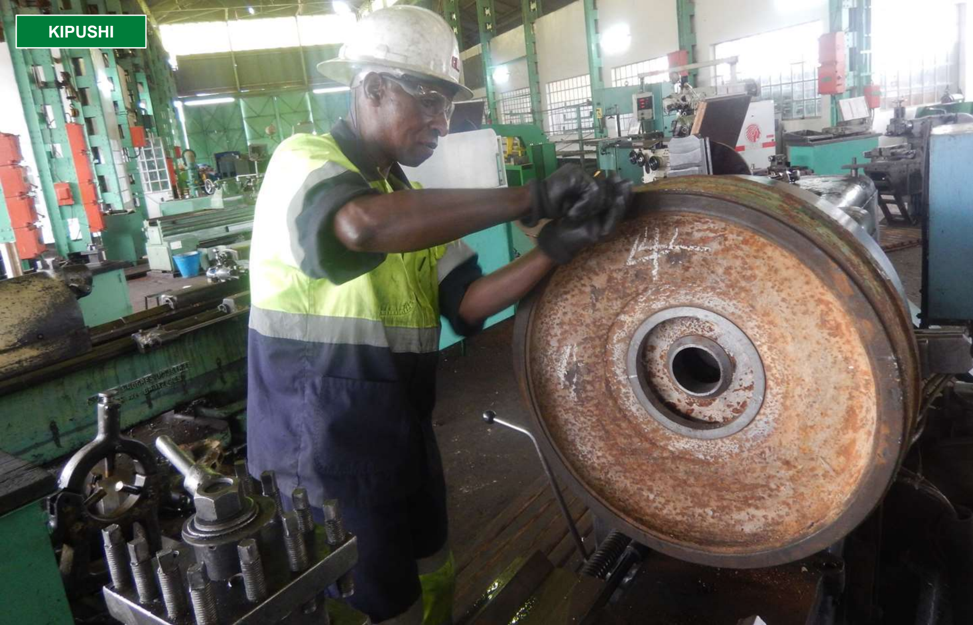
Raymond Mutumbwe working on a diaphragm plate for a pump that will be installed at the 710-metre-level station.
