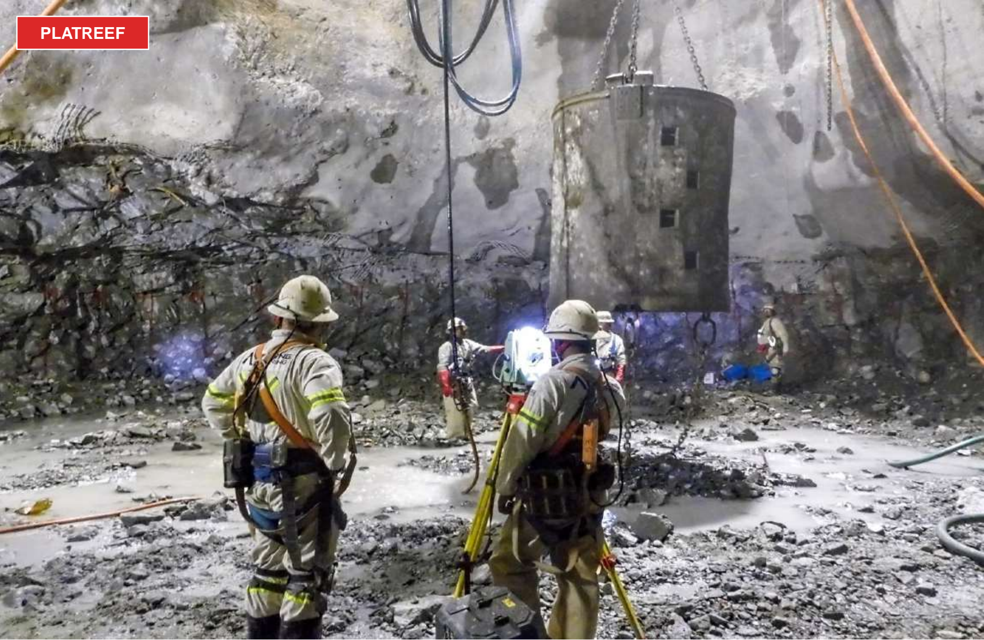
Engineers surveying Shaft 1's 950-metre-level station. The kibble (bucket), used for hoisting broken rock to surface, is positioned for filling.
