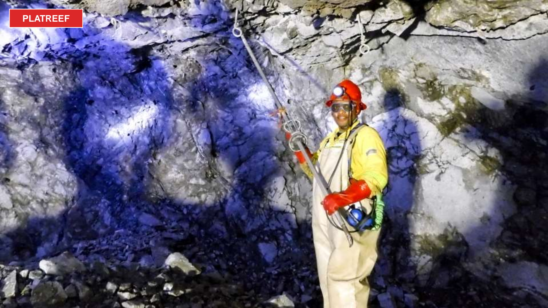
Lesetsi (Rock Drill Operator) conducting rock scaling following a blast at the 950-metre-level station.
