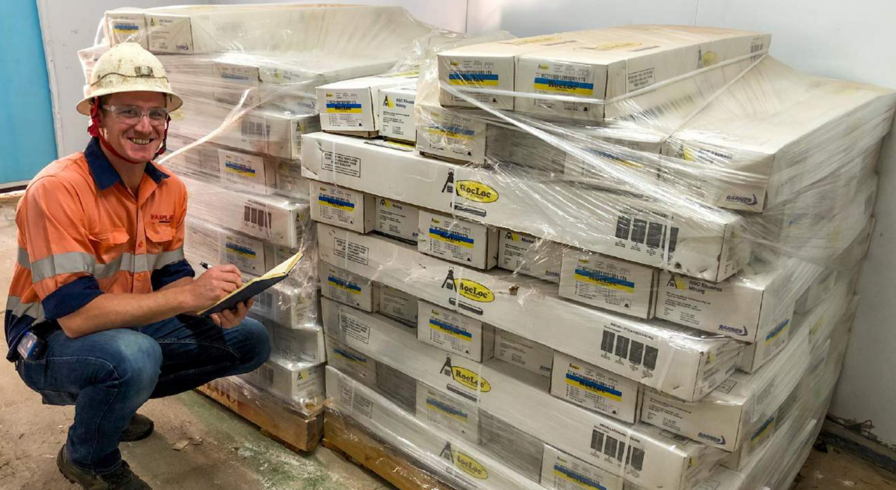
Tim Hudson, Acting Rock Engineer, inspecting a delivery of resin capsules at Platreef's Shaft 1. The resin is being used to grout and seal rock anchor bolts at the 950-metre station, helping to ensure safe and productive mining operations.
