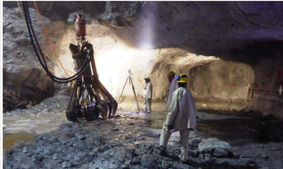
Members of Platreef’s underground mining team using a “cactus grab” mucker to excavate rock from the bottom of Shaft 1
