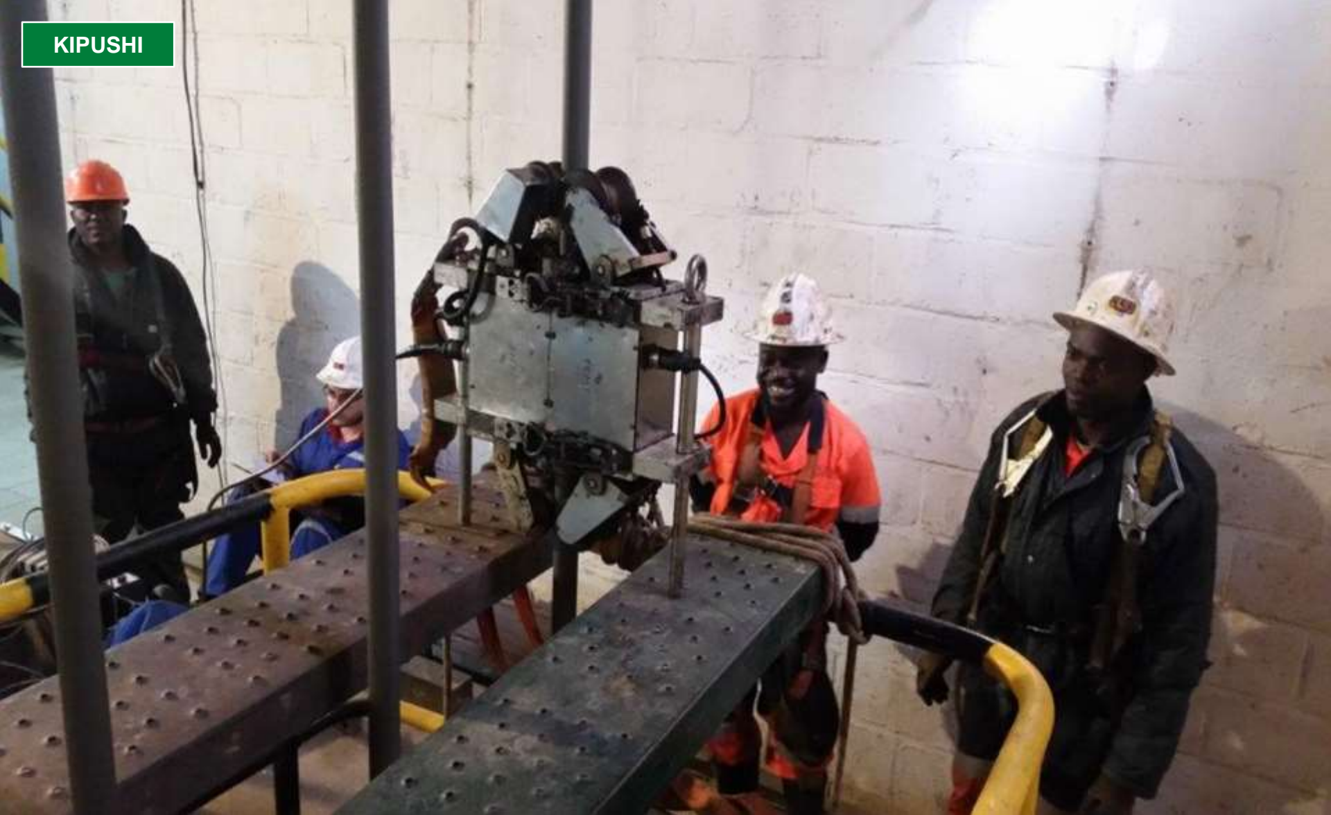
Kipushi's engineering team conducting electro-magnetic testing of the steel cables (ropes) on the mine's drum winders.
