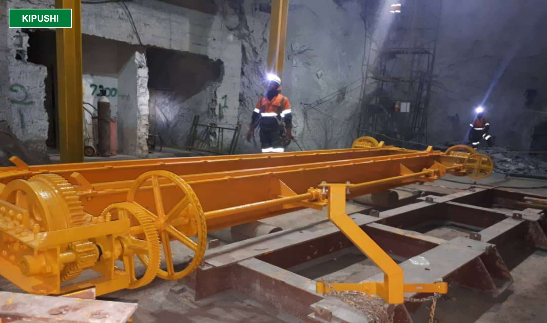
Refurbished and newly painted overhead crane at Kipushi's 850-metre-level pump chamber.
