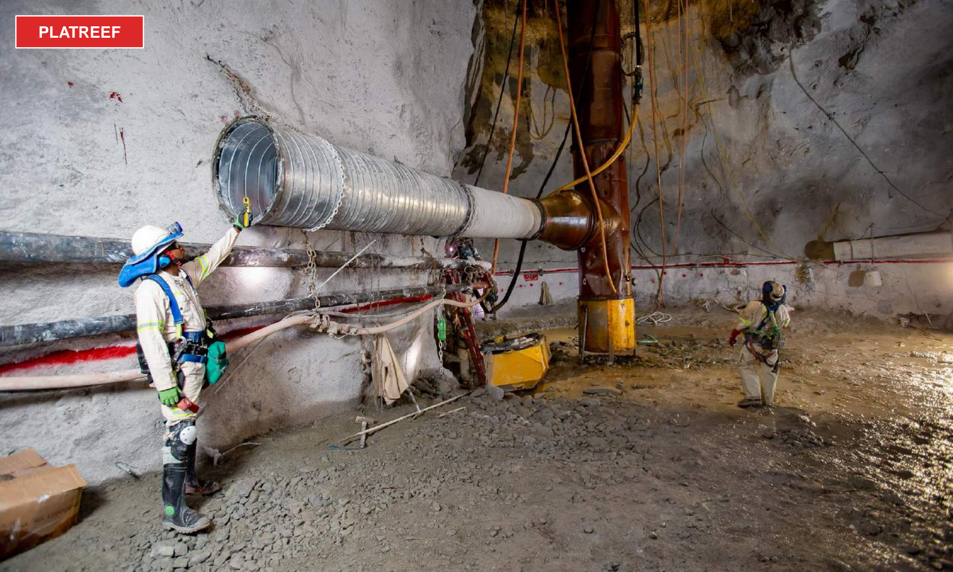
Jan Mojabelo, Ivanplats' Ventilation Officer, measuring the flow of fresh air coming from surface to Shaft 1's 850-metre-level station.
