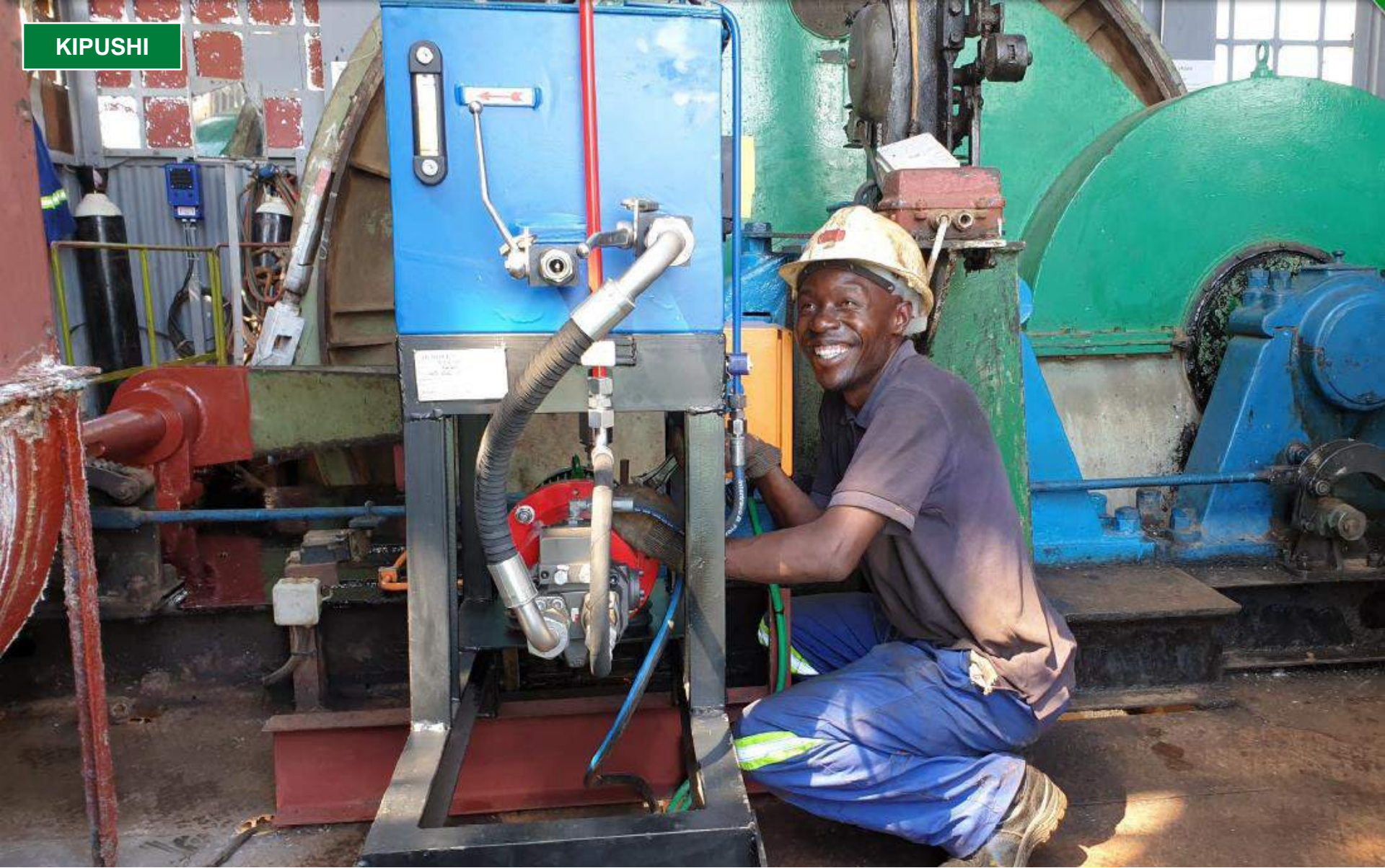
Kahudi Mununga connecting up a new hydraulic power pack for the brakes on the P3 hoist.
