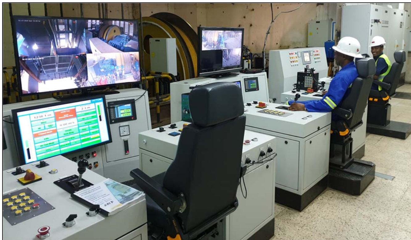
Photo: Modern, new control room at Kipushi's Shaft 5.
