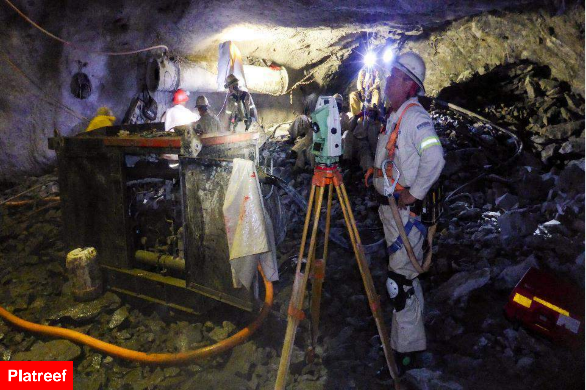
An engineer surveying the ongoing lateral development work at Shaft 1's 850-metre-level station.
