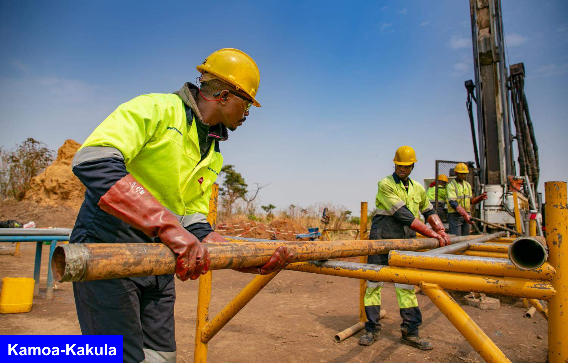
Exploration drillers collecting a core sample from a drill rod at Kamoa North.
