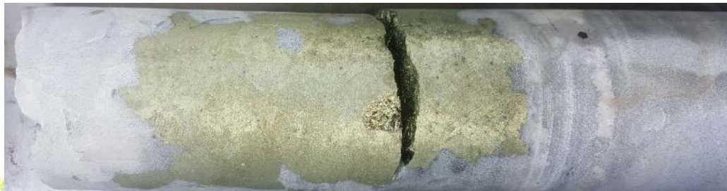
Above: Recent Kakula drill core showing massive chalcopyrite mineralization within a carbonate vein.
