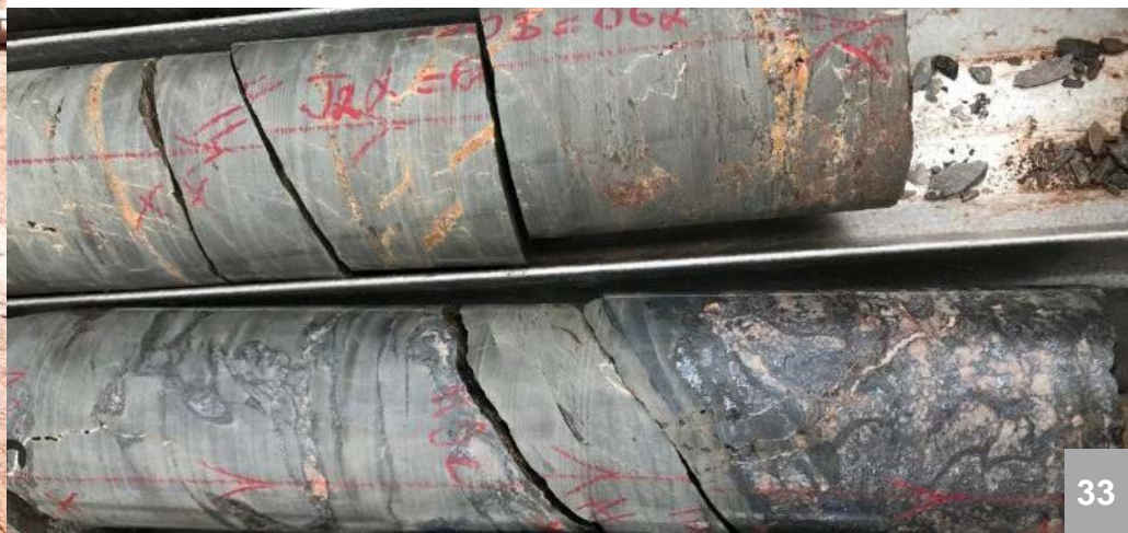
Below: Massive and bedded chalcocite within siltstone.
