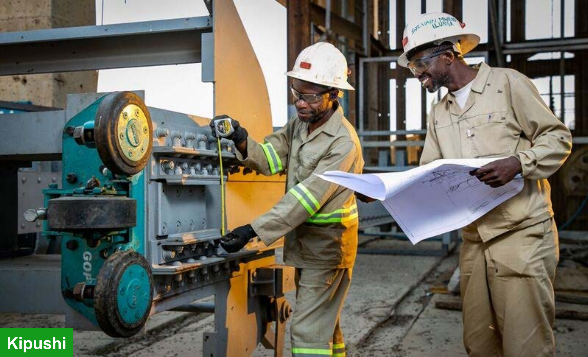
Ilunga Mwamba and Mwendi Ilunga installing wheels onto a carrying frame, or bridle, for Kipushi's underground rock winder, prior to it being lowered down Shaft 5.
