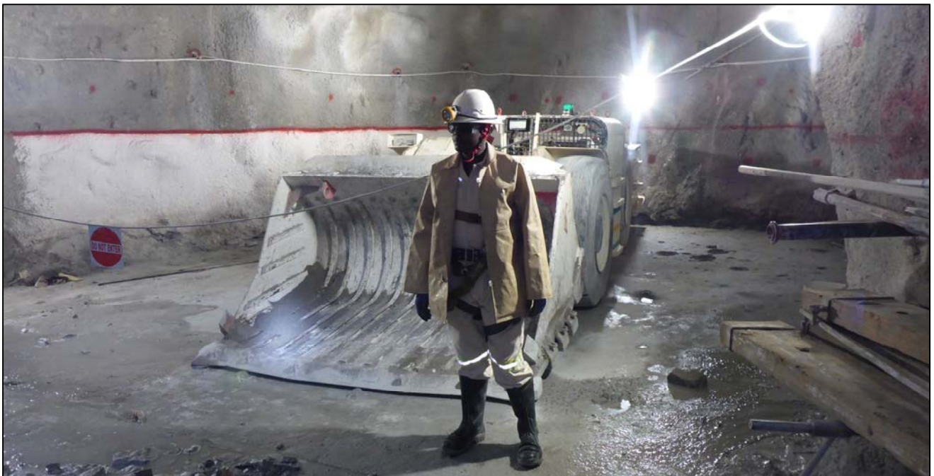
Figure 2: An equipment operator with Platreef's 5.5-tonne, load-haul-dump machine used for excavating the 750-metre station.
