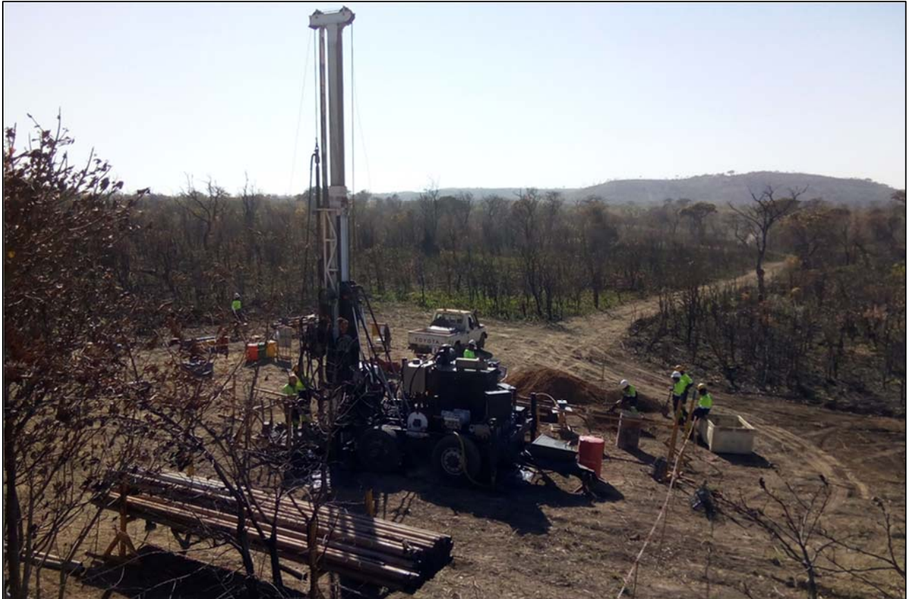
Figure 12: Exploration drilling testing a zone of strong copper mineralization at Kamoa North.
