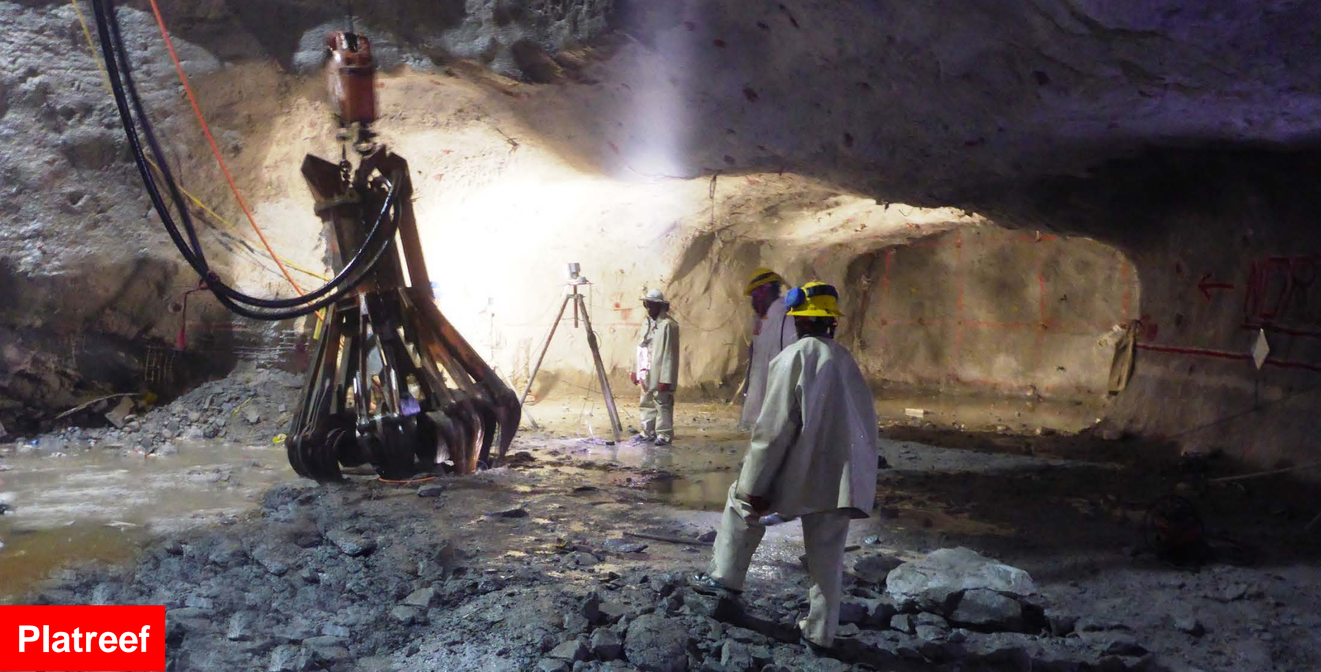
Member of Ivanhoe's Platreef shaft-sinking team with a cactus grab used to remove excavated rock from lateral mine development on the 750-metre level of Shaft 1.
