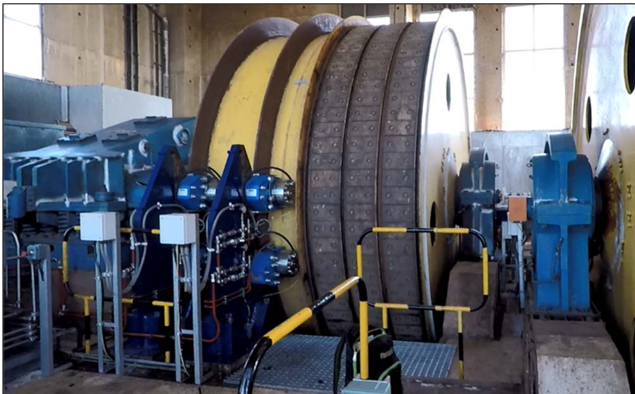
Figure 5: The fully-commissioned rock winder. All of the rock winder's safety and drive systems have been successfully tested to international standards.
