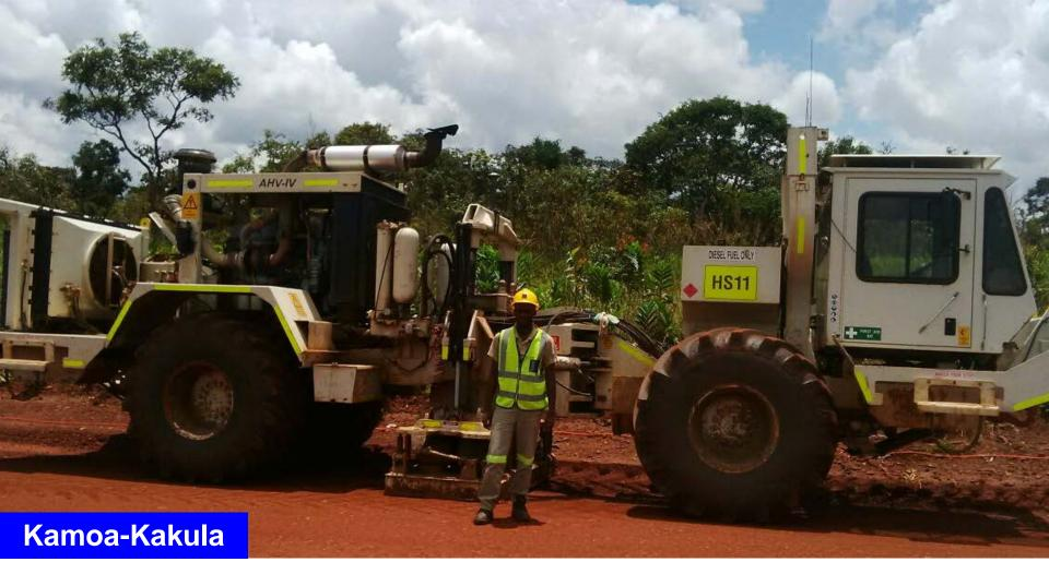
Geologist Nestor Kambaj at a mobile, seismic vibrator rig being used by Hi-Seis, a leading international services company, to survey the Kamoa-Kakula licence area. The device creates seismic waves to produce reliable, quality images of hard-rock environments to help identify drilling targets to test for potential, Kakula-like discoveries.
