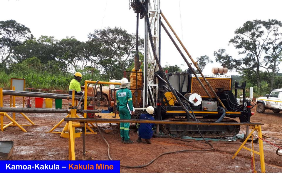
One of 13 rigs at the Kakula Discovery. More than 21,000 metres have been drilled since the beginning of 2018, including step-out holes to expand the resources, in-fill holes to upgrade the resources, and wedge holes for metallurgical test work.
