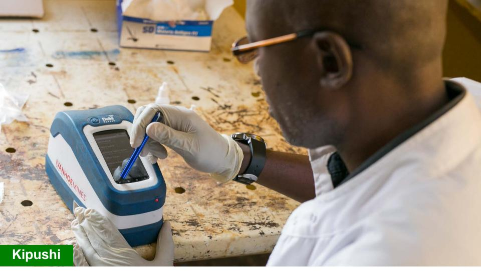
Deki devices provide automated readings of rapid diagnostic tests, removing the human-error factor and avoiding unnecessary prescription of medication, as part of the Ivanhoe-sponsored Fionet program to improve malaria diagnostics and treatment in Haut-Katanga and Lualaba provinces, in southern DRC, which host Ivanhoe's Kipushi and Kamoa-Kakula projects..
